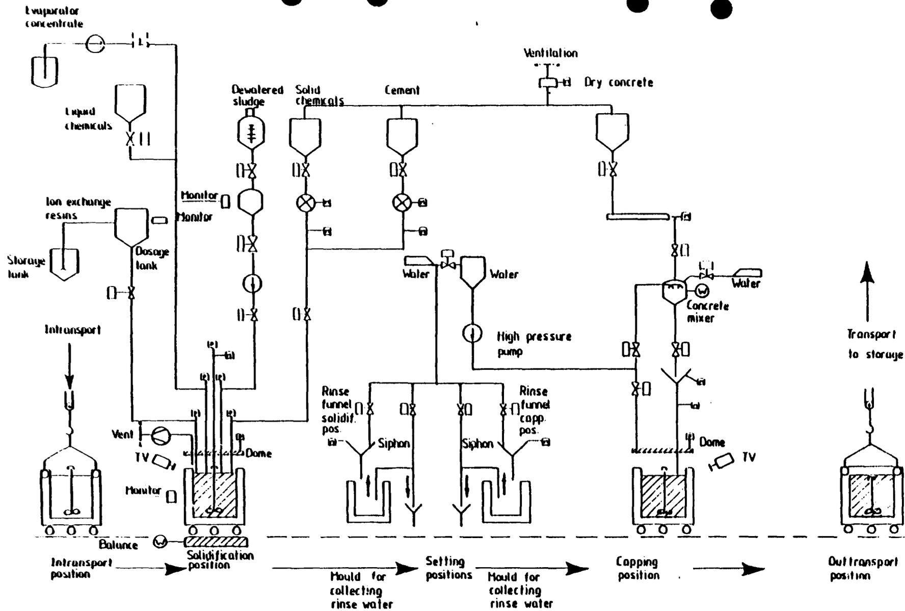
Figure 3 ASEA-ATOM - RINGHALS CONCRETE SOLIDIFICATION SYSTEM
