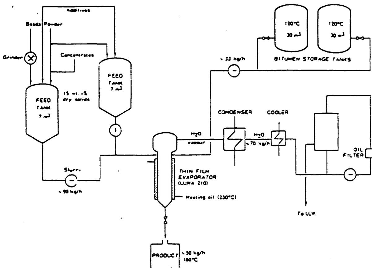
Figure 4 Bituminisation of spent resins at the Barsebeck nuclear power plant.
