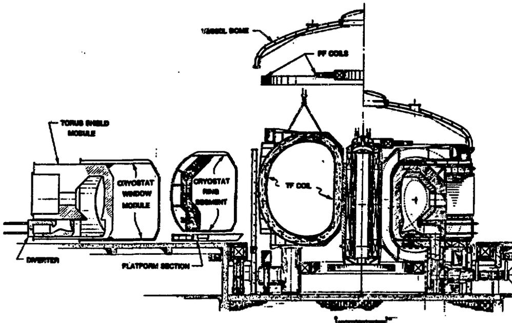
FIGURE 3: TF COIL REPLACEMENT APPROACH SHOWING WHICH COMPONENTS MUST BE REMOVED TO GAIN ACCESS TO THE COIL
