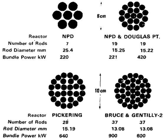
Figure 3 Cross sections of CANDU power reactor fuel bundles.
