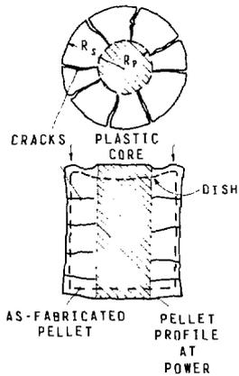
Figure 5 Schematic diagram showing how a fuel pellet expands.
