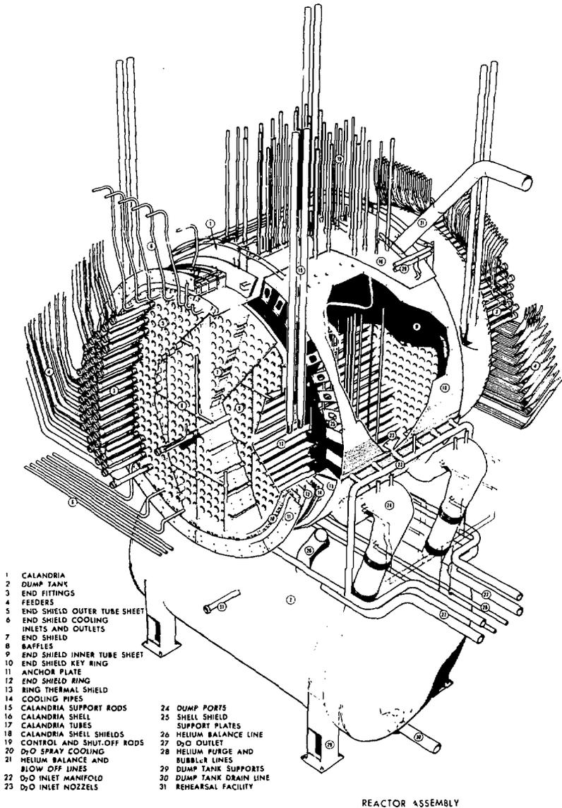
Figure 1 CANDU Reactor, showing the array of horizontal pressure tubes passing through the calandria.
