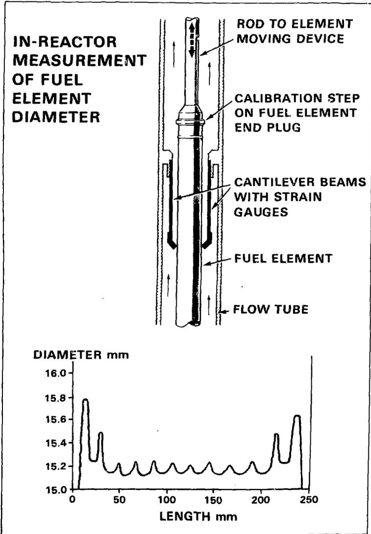
Figure 6 Schematic illustration showing the IRDMR measuring a fuel element diameter in a pressurized water loop (10).
