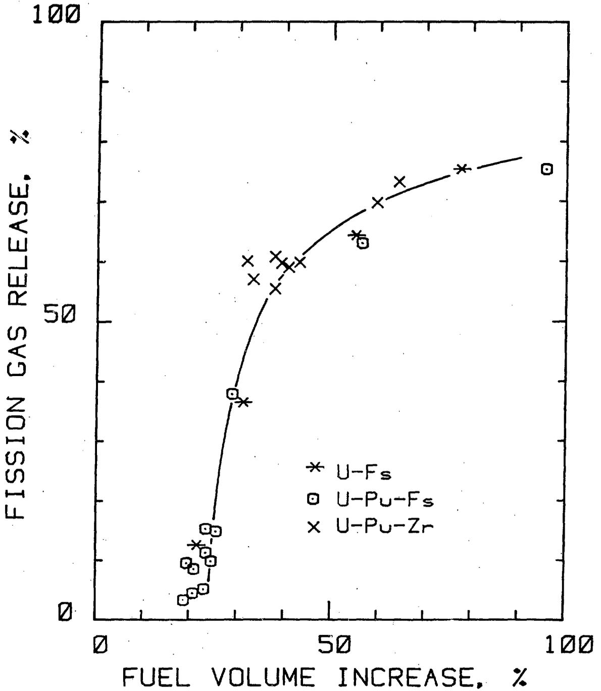
Figure 1. Effect of fuel swelling on fission-gas release in metal fuels.
