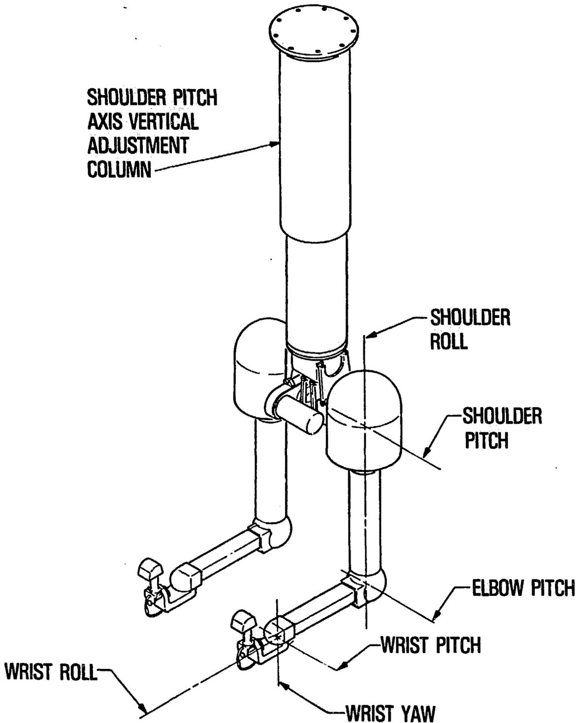
Fig. 3. Advance servomanipulator master arm.
