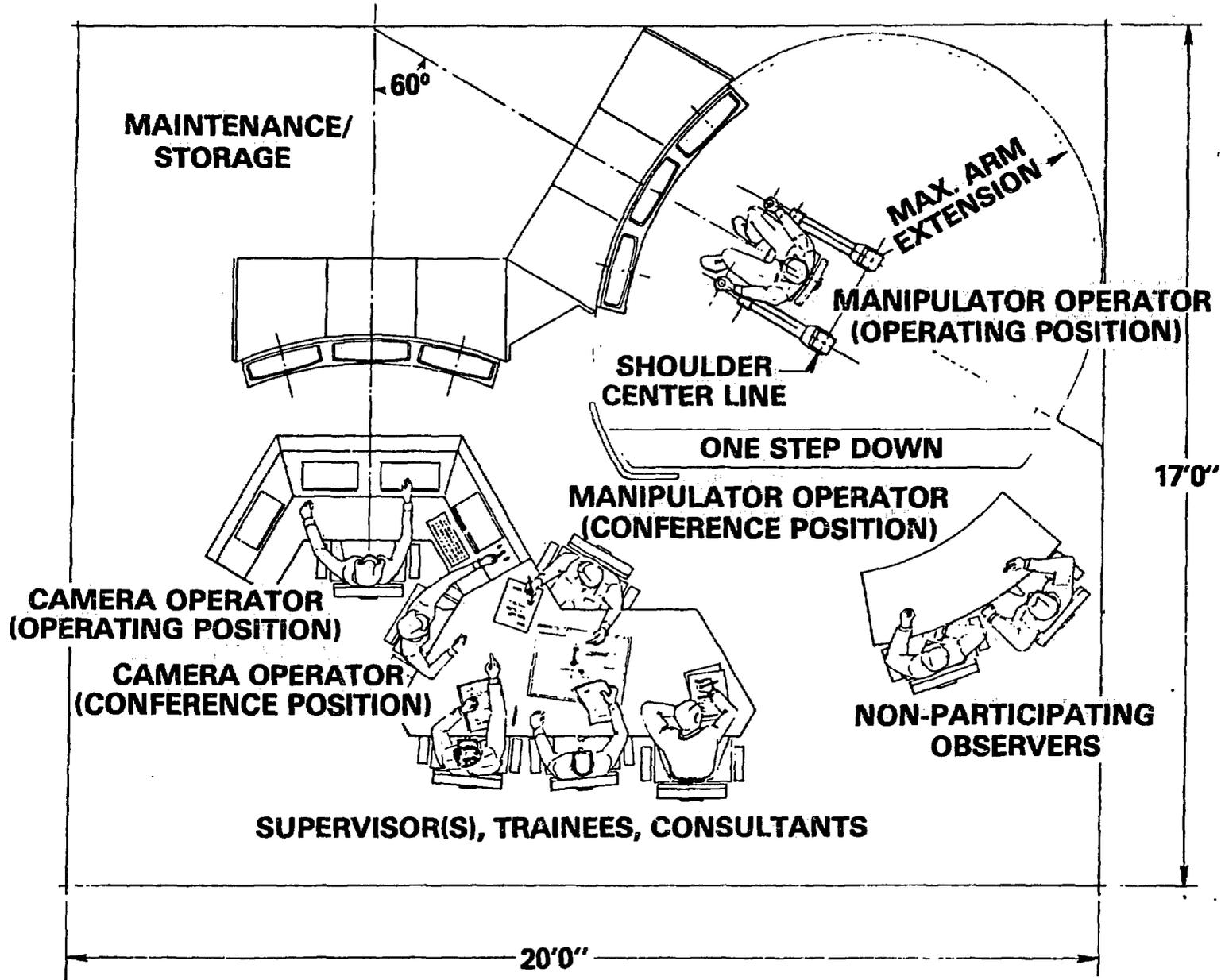
Fig. 2. Integrated operator control station: Plan View
