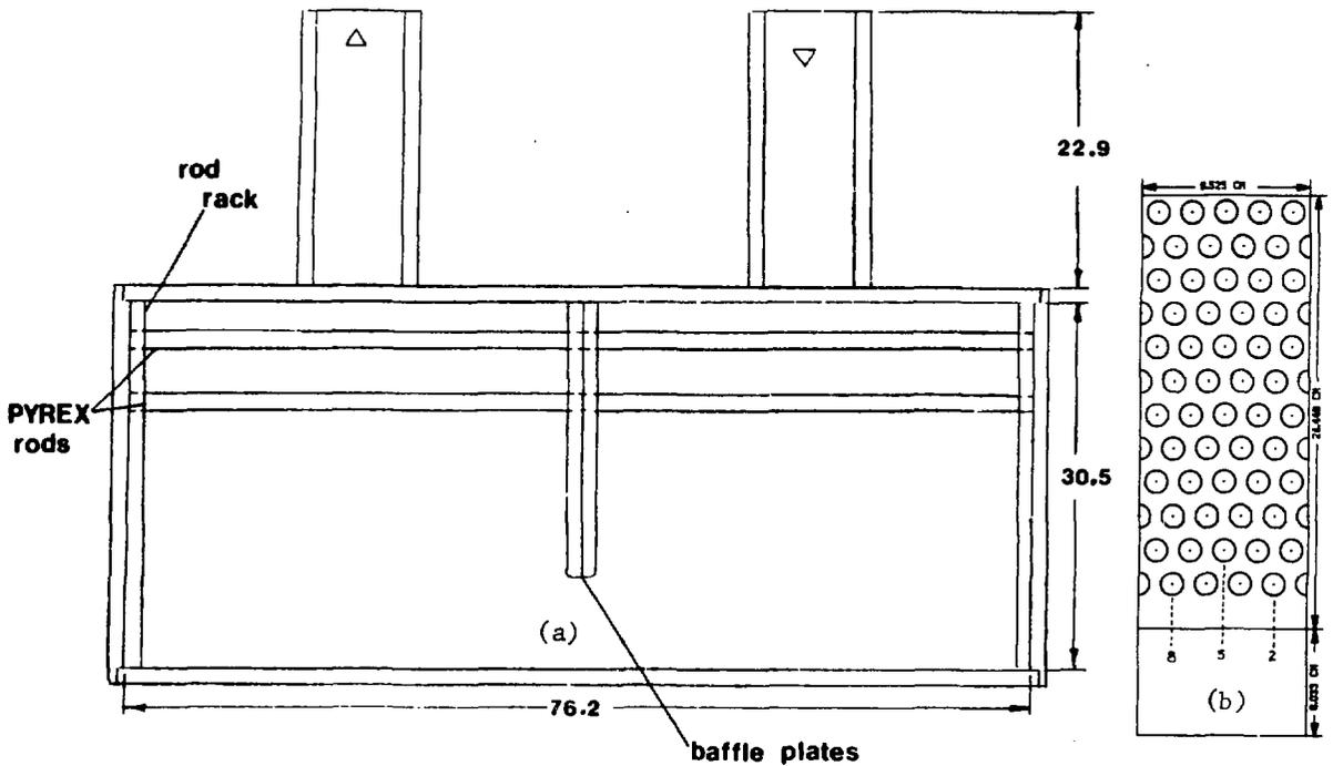
FIGURE 1: Heat Exchanger Model-(a) Front View, (b) End View Showing the Three Measuring Planes 2,5 and 8.
