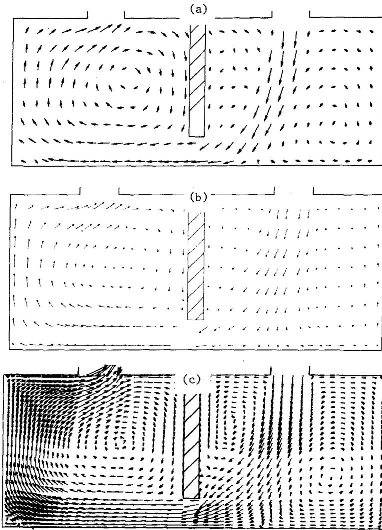
FIGURE 4: Velocity Distributions For The Tube-Free Model-(a)Measured, (b) Coarse Grid Prediction, (c) Fine Grid Prediction
