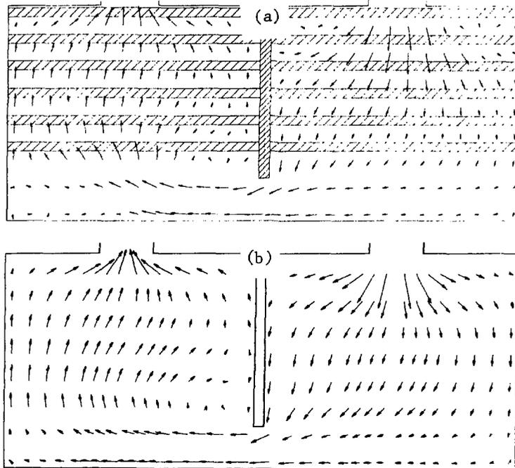
FIGURE 3: Velocity Distributions for the Tube-Filled Model With Tube-to-Baffle Leakage-(a) Measured, (b) Predicted
