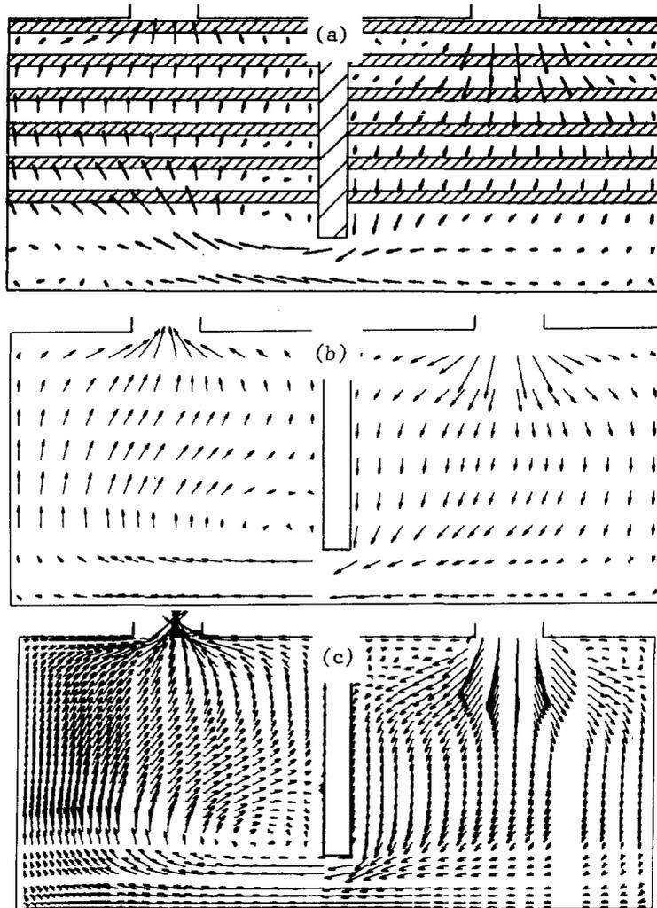
Figure 2: Velocity Distributions for the Tube-Filled Model With No-Leak Baffle-(a) Measured, (b) Coarse Grid Prediction, (c) Fine Grid Prediction; 1 cm=2.25 m/s in All Plots
