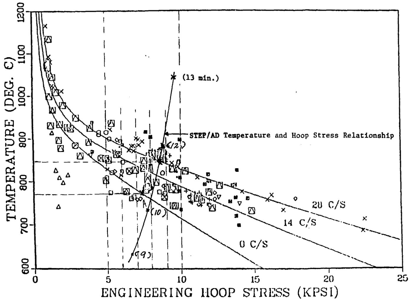
F Fig. 1. STEP/AD Clad Temperature and Hoop Stress Behavior Versus Experimental Data
