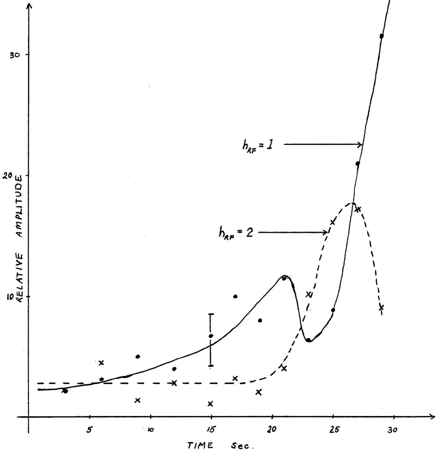
Fig. 7 Plot of  $h = 1$  and  $h = 2$  FFT moments of protons cooling into a bucket as a function of time. Two  $\sigma$  error bars (500 particles) are indicated.
