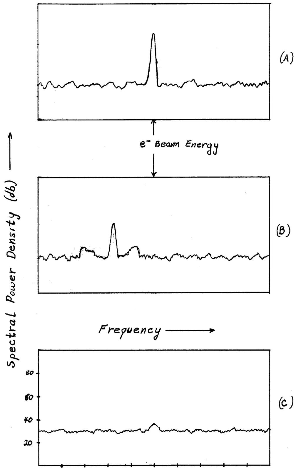
Fig. 4 a) tuned ( $E_e \rightleftharpoons \omega_{RF}$ ) case: peak is at  $60 \omega_{RF} = 453.97$  MHz. Trace is 16 KHz/Div. b)  $\omega_{RF}$  detuned by -310 Hz. c)  $\omega_{RF}$  detuned > 1 KHz.
