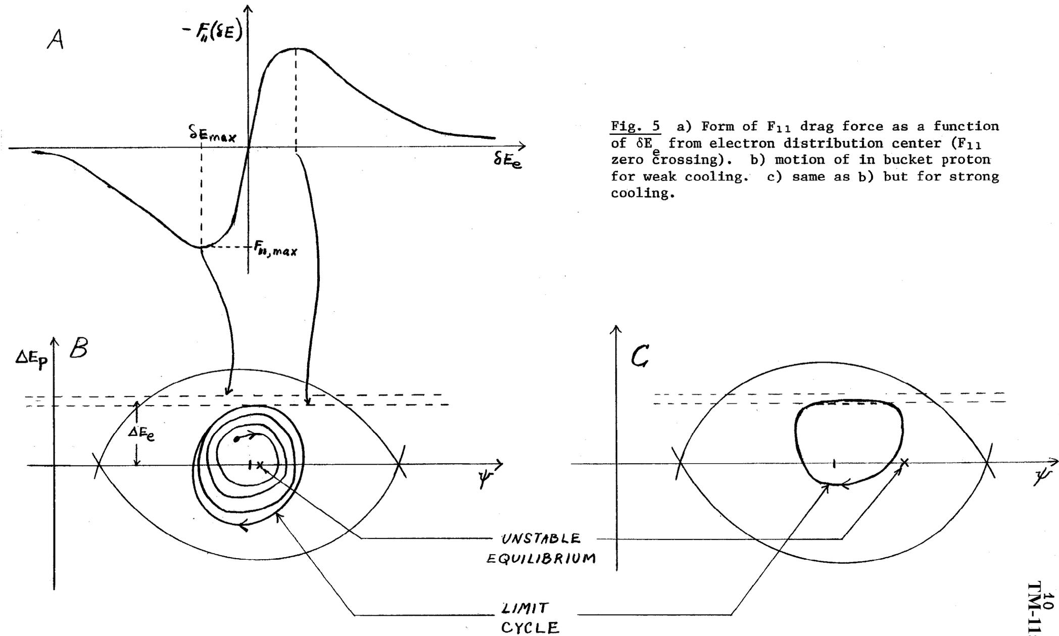
Fig. 5 a) Form of  $F_{11}$  drag force as a function of  $\delta E_e$  from electron distribution center ( $F_{11}$  zero crossing). b) motion of in bucket proton for weak cooling. c) same as b) but for strong cooling.
