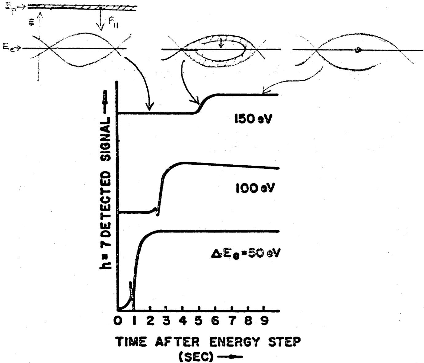
Fig. 3 Time sequence of a narrow momentum spread proton band (cold) being dragged into an R.F. bucket. Three experimental traces are illustrated (with different initial offsets). The transient at capture is to be noted.
