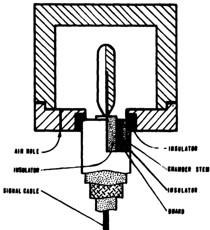
Fig. 1 - Scheme of the graphite cavity chamber.
