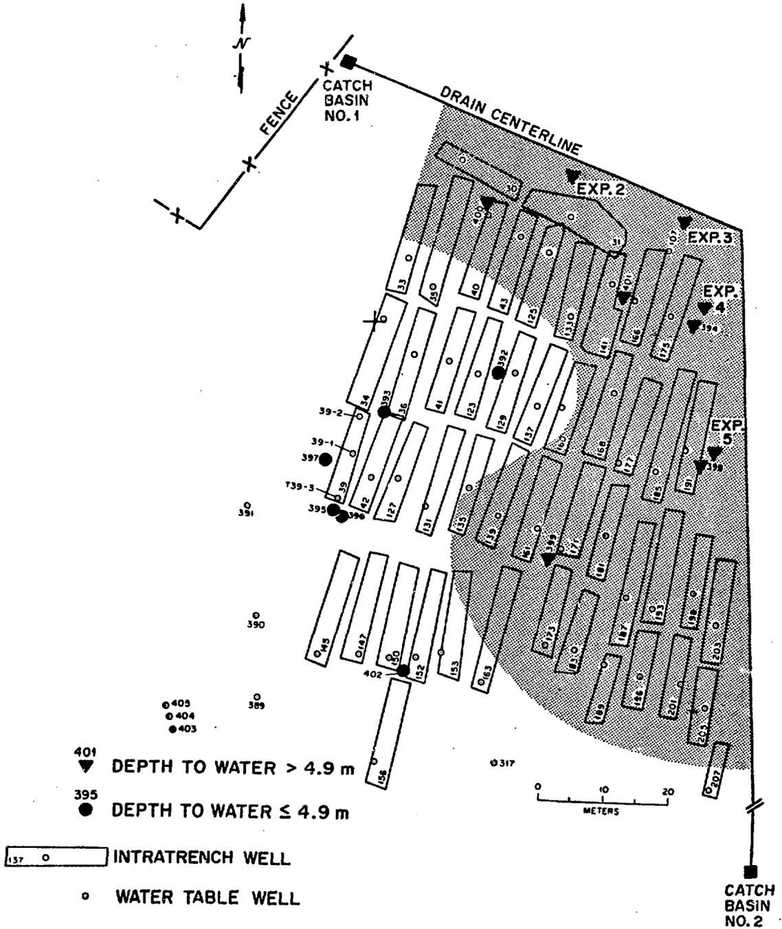
Figure 3. Plan view of the 49-Trench area showing region of groundwater suppression.
