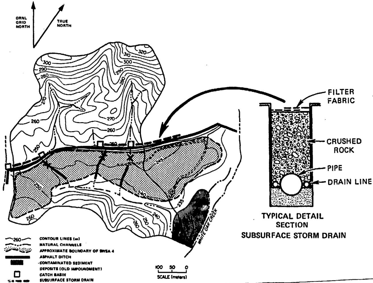
Figure 2. Location of the surface water diversion project within ORNL Solid Waste Storage Area 4.
