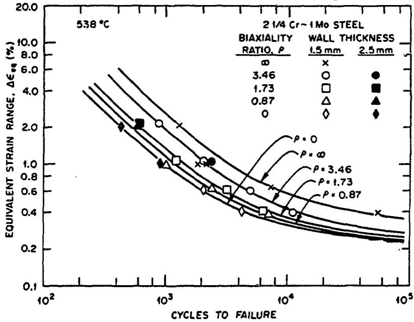
Fig. 10. Mises equivalent strain range vs cycles to failure for multiaxial fatigue tests of 2-1/4 Cr-1 Mo steel tubes at 538°C. ( $\rho = 0$  corresponds to uniaxial straining;  $\rho = \infty$ , to pure torsional straining.)
