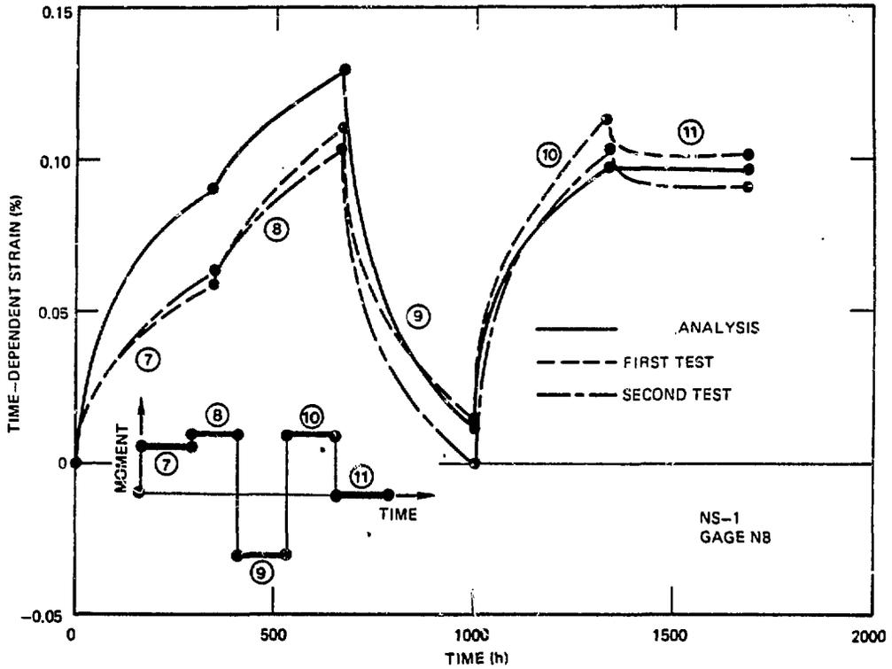
Fig. 5. Time-dependent circumferential strain measurements and predictions for two repeated moment-only tests of a nozzle-to-spherical shell specimen (transition region behavior).
