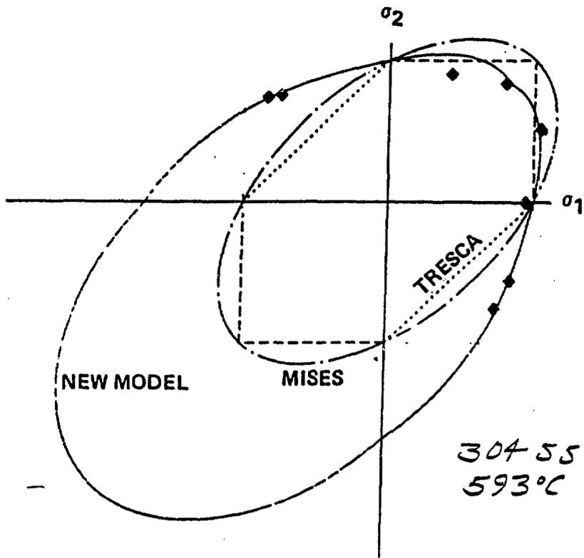
Fig. 9. Biaxial isochronous stress rupture contours showing that new creep-rupture criterion fits 304 stainless steel data much better than the classical criteria.
