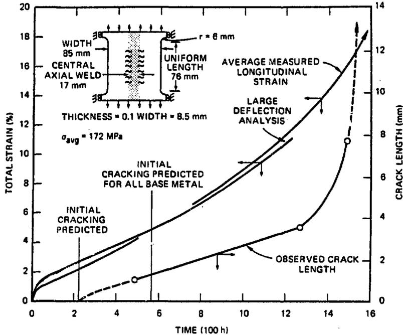
Fig. 3. Comparison of analytical predictions with experimental results for typical 304/308-CRE plate weldment creep-rupture test performed by Westinghouse.
