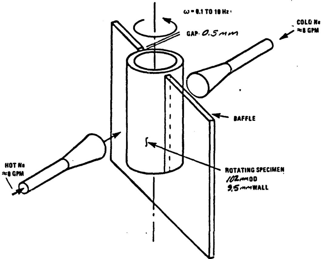
Fig. 11. Conceptual representation of Westinghouse thermal striping test concept, based on rotating cylinder specimen.
