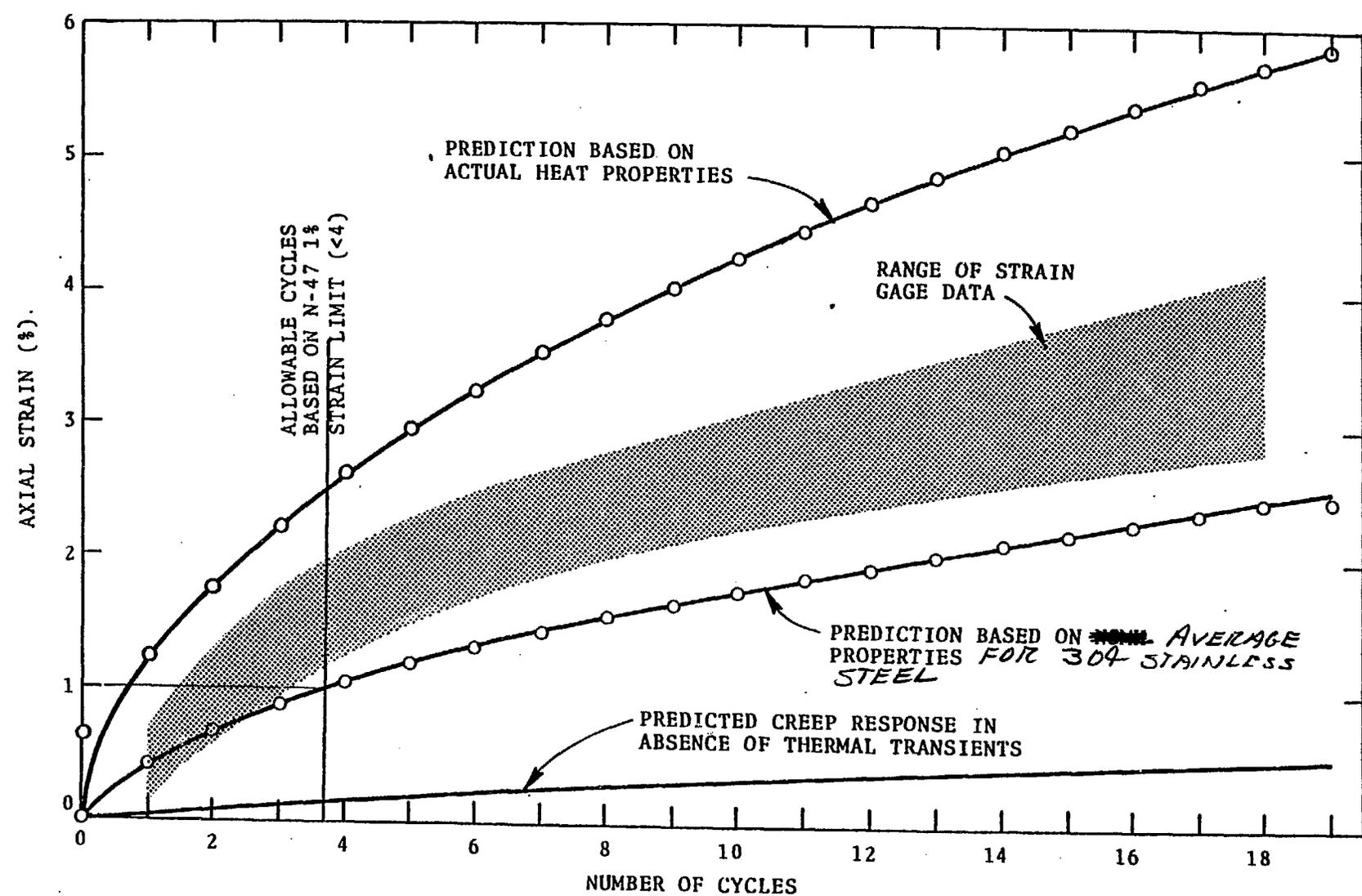
Fig. 7. Measured vs predicted axial ratchetting strain on outer surface of type 304 stainless steel pipe thermal ratchetting specimen.
