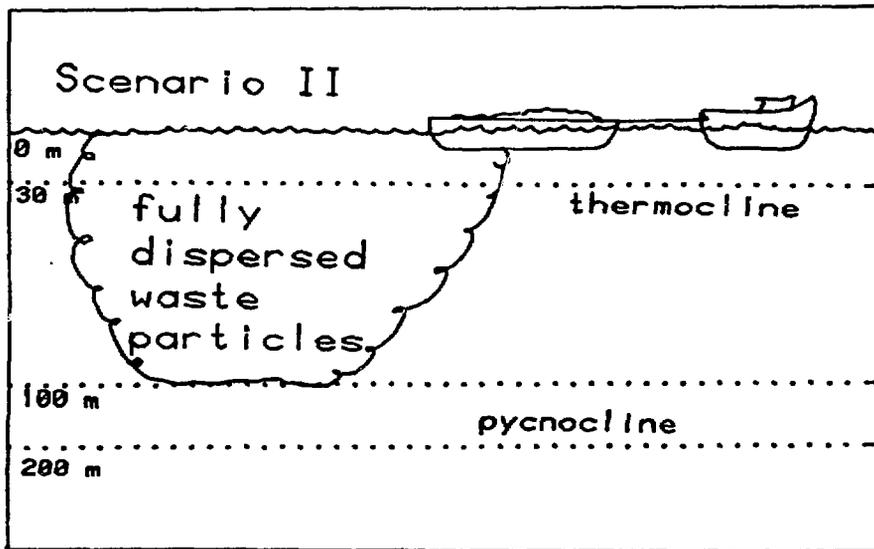
Figure 2. Schematic Diagram of Two Bounding Scenarios Used for Assessment of Impacts from Ocean Disposal of the NFSS Wastes. Source: U.S. Department of Energy (1984).
