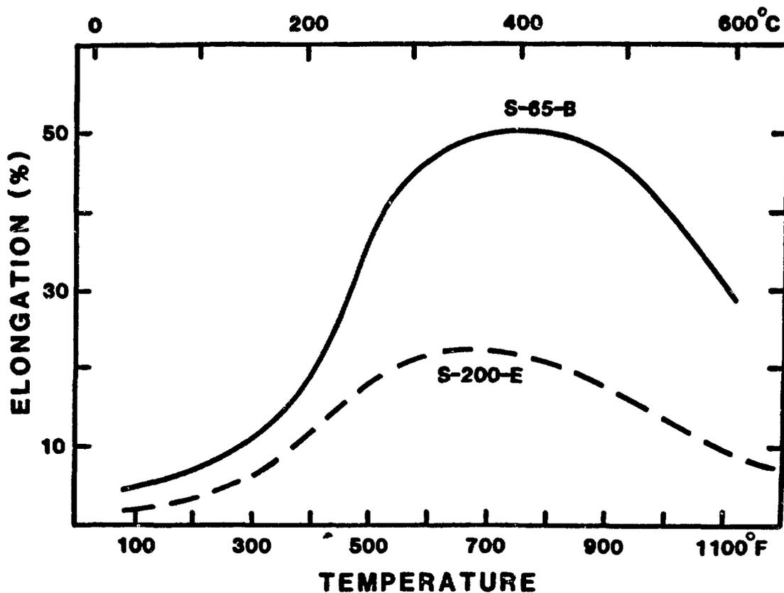
Fig. 4. Measured values of ductility as a function of temperature for two grades of beryllium.
