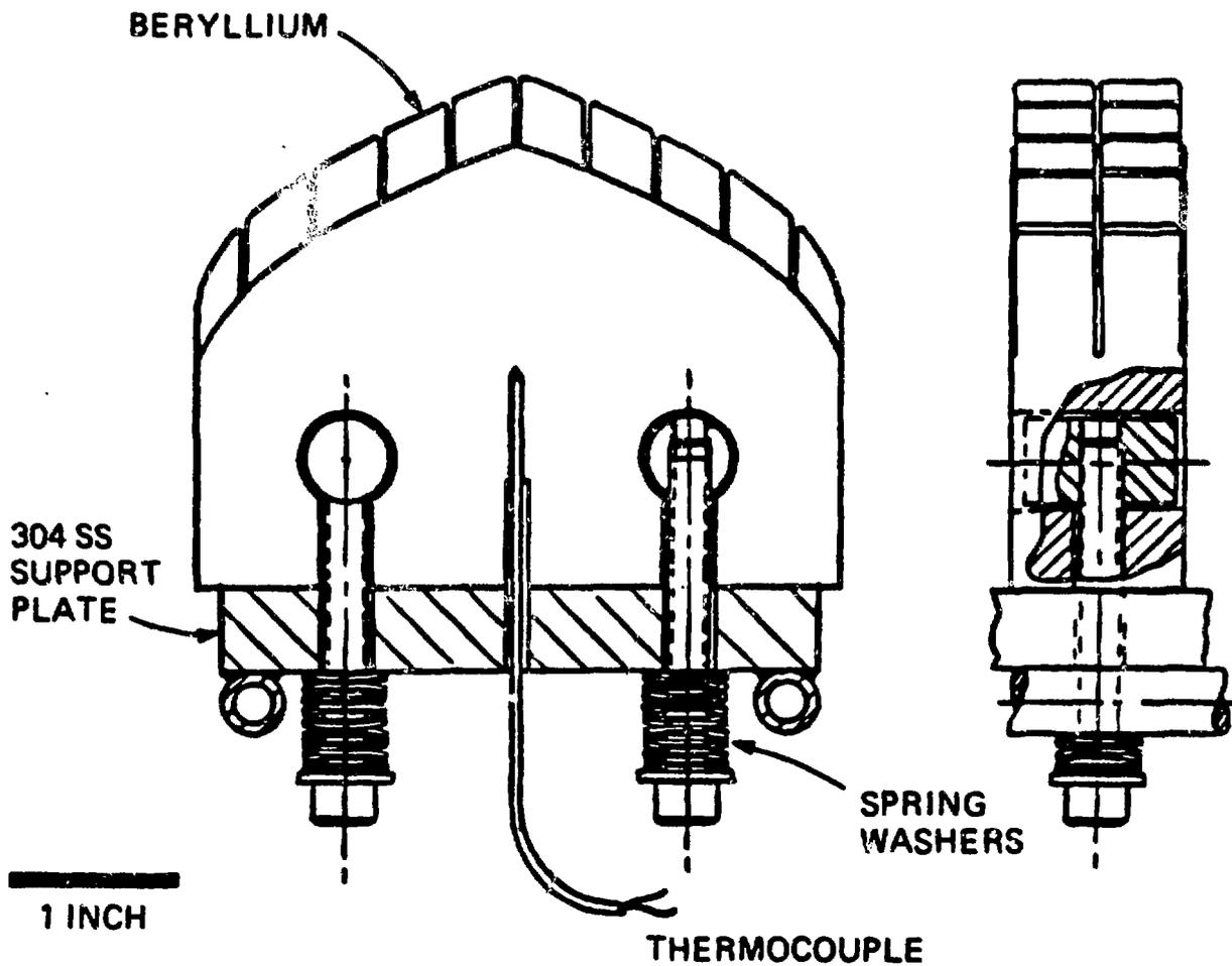
Fig. 2. Drawing of tessellated beryllium limiter tile showing mounting details.
