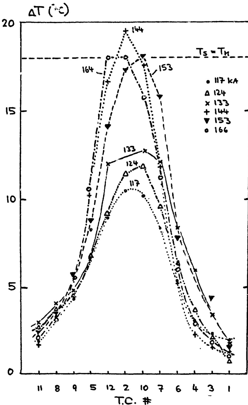
Fig. 7. Limiter temperature and energy distribution as function of plasma current for NBI heated discharges (PB=0.85 MW)
