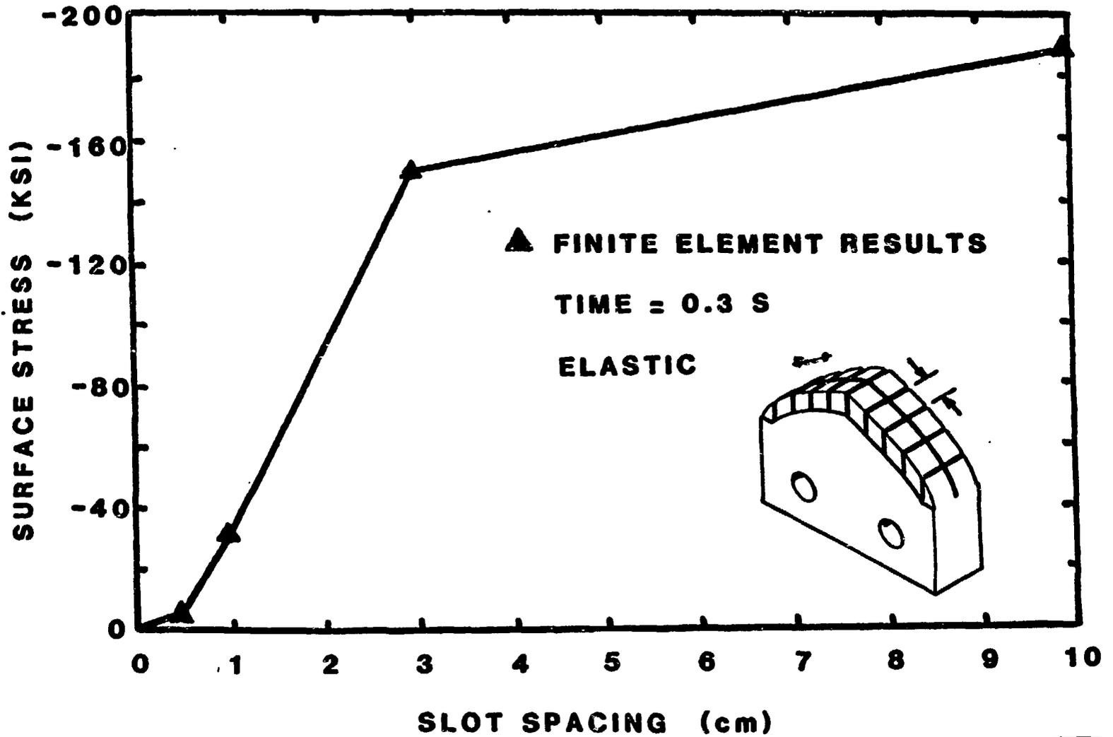
Fig. 3. Effect on surface stress and changing slot spacing (model assumes 2.5 kN/cm<sup>2</sup> for 0.3 sec.)
