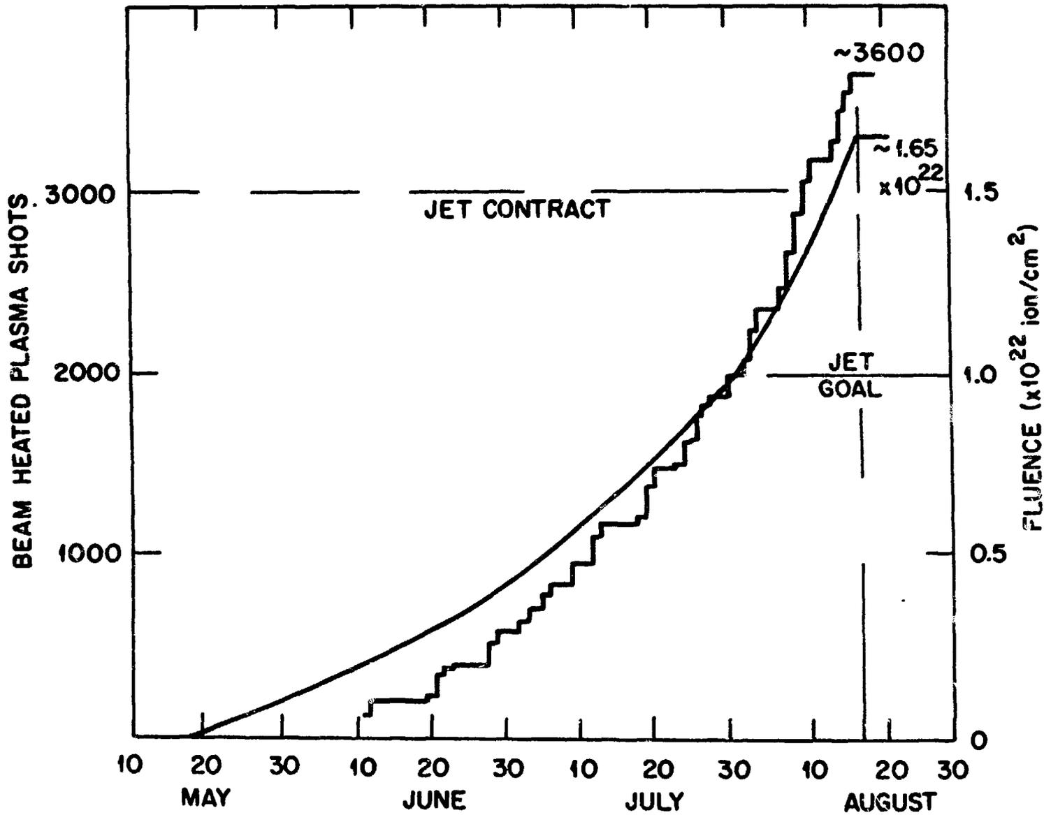
Fig. 6. Graph of beam heated shots and estimated limiter fluence during beryllium limiter experiment.
