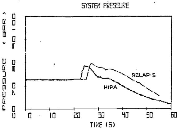
Figure 9. Comparison of Plant Analyzer Results with RELAP-5 Calculations for Failure of Feed-water Controller at Maximum Demand, System Pressure
