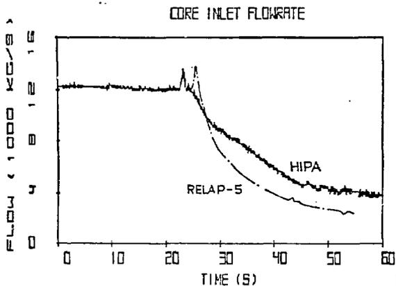
Figure 10 Comparison of Plant Analyzer Results with RELAP-5 Calculations for Failure of Feed-water Controller at Maximum Demand, Core Inlet Mixture Mass Flow Rate
