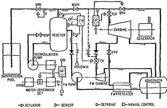
Figure 1 BWR Plant Schematic
