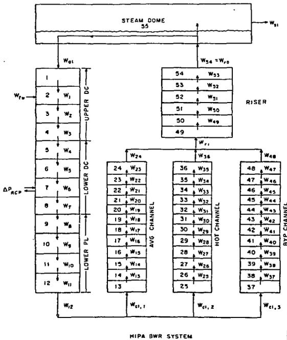
Figure 2 Vessel Flow Schematic and Arrangement of Computational Cells in Pressure Vessel
