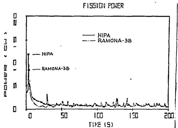
Figure 7 Comparison of Fission Power Predictions from Plant Analyzer and RAMONA-3B Code
