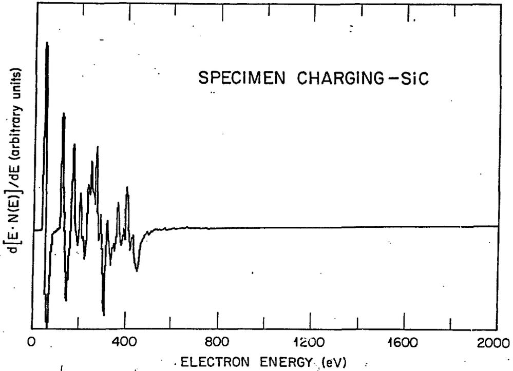
Fig. 9. Typical secondary electron spectrum from an electrically insulating specimen exhibiting charging.
