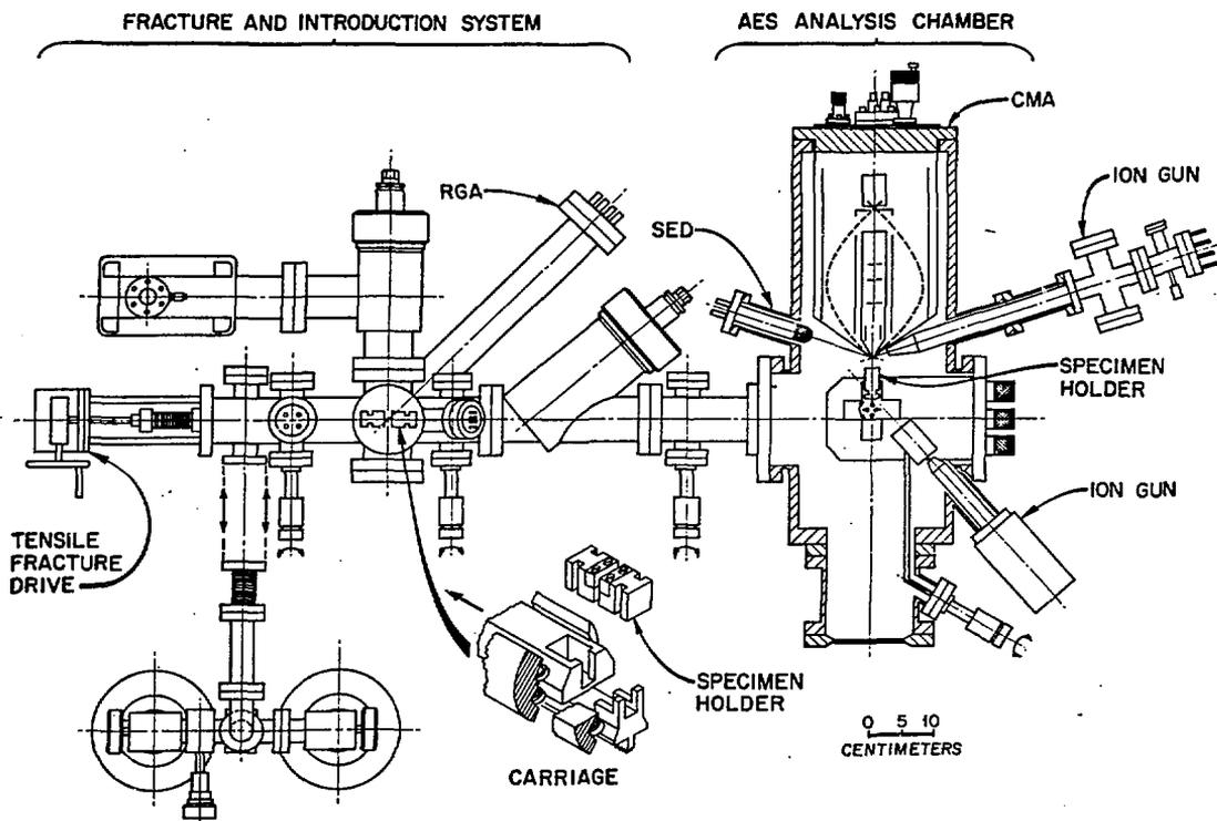
Fig. 8. Schematic view of a more complex AES system, based on the analysis chamber in Fig. 7.
