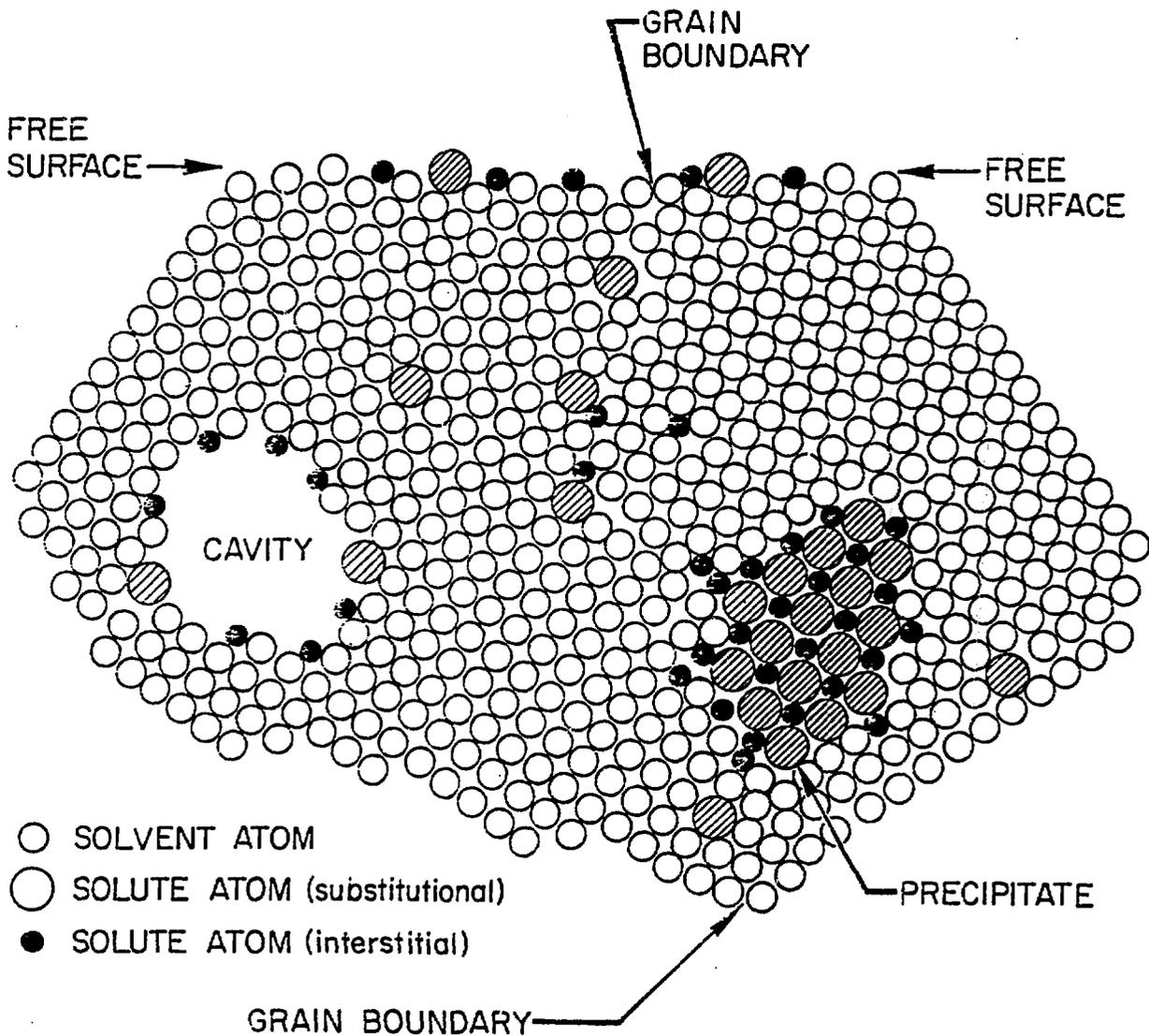
Fig. 1. Schematic illustration of the various types of interfaces that may exist in crystalline materials.
