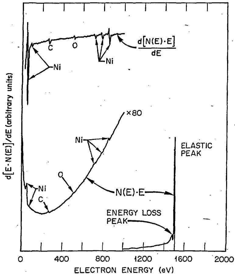
Fig. 4. Secondary electron spectra from a Ni alloy, obtained using a cylindrical mirror analyser (CMA).
