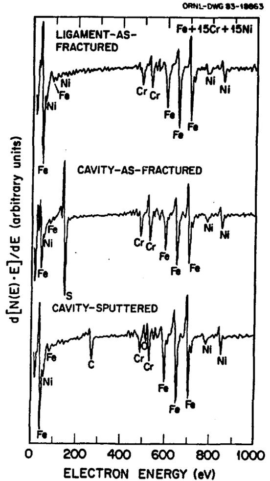
Fig. 6. Conventional scanning electron micrograph (a), secondary electron image (b), sulfur map (c) and Auger spectra (d) of a creep cavitated austenitic steel that was fractured in the AES analysis chamber to expose creep cavity surfaces [B in (b)] and transgranular rupture of intercavity ligaments [A in (b)].
