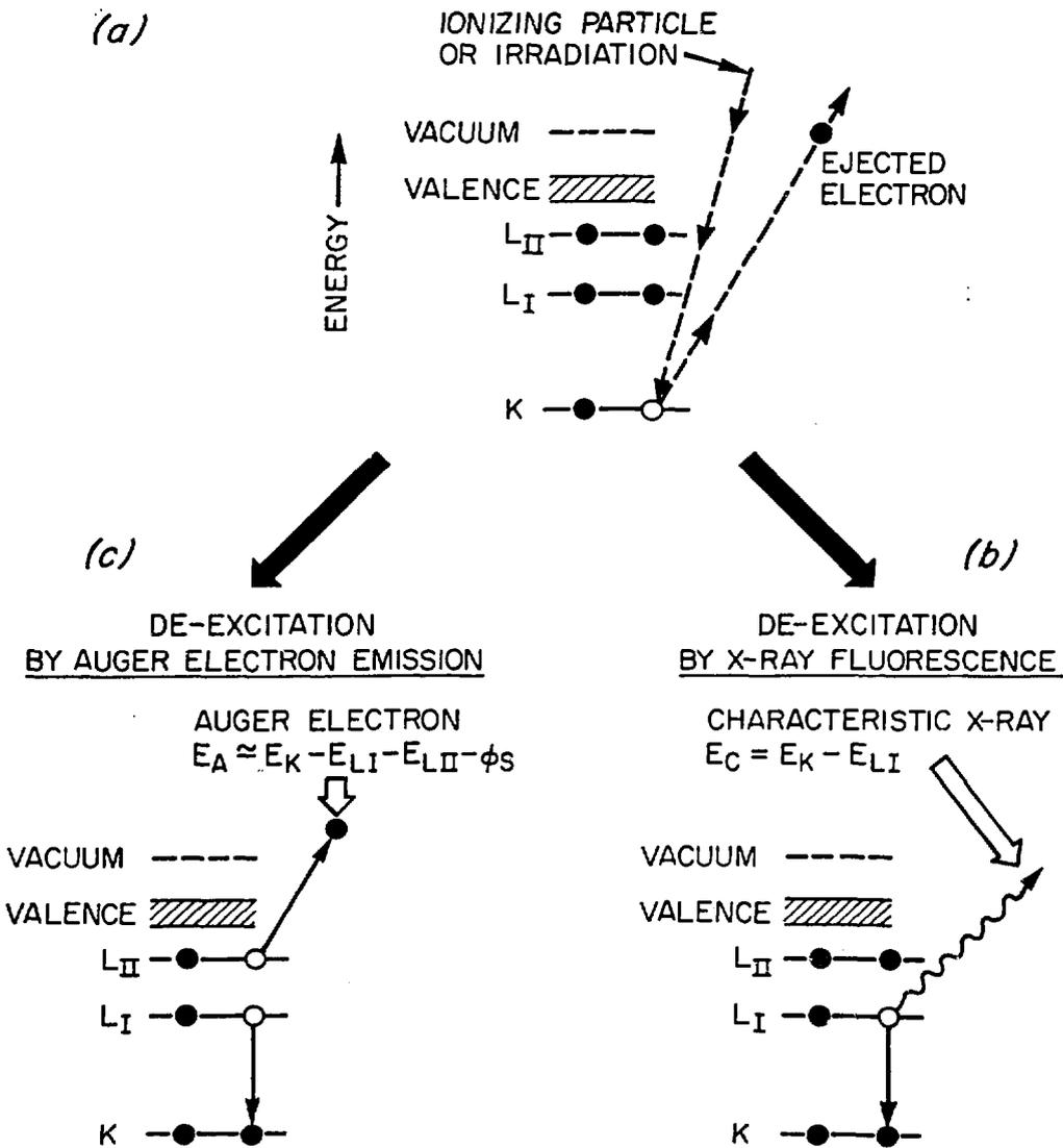
Fig. 3. Comparison of the Auger transition with the more familiar process of x-ray fluorescence.
