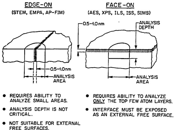
Fig. 2. Schematic illustration showing two distinct modes of interfacial analysis.
