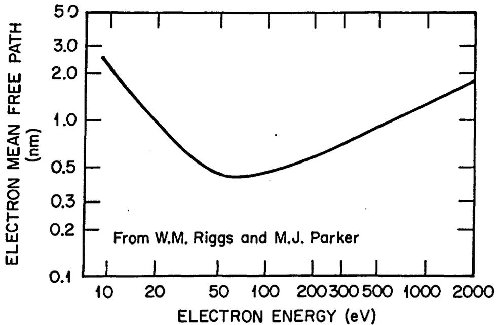
Fig. 5. Plot of the inelastic electron mean free path as a function of electron energy, after Riggs and Parleer (24).
