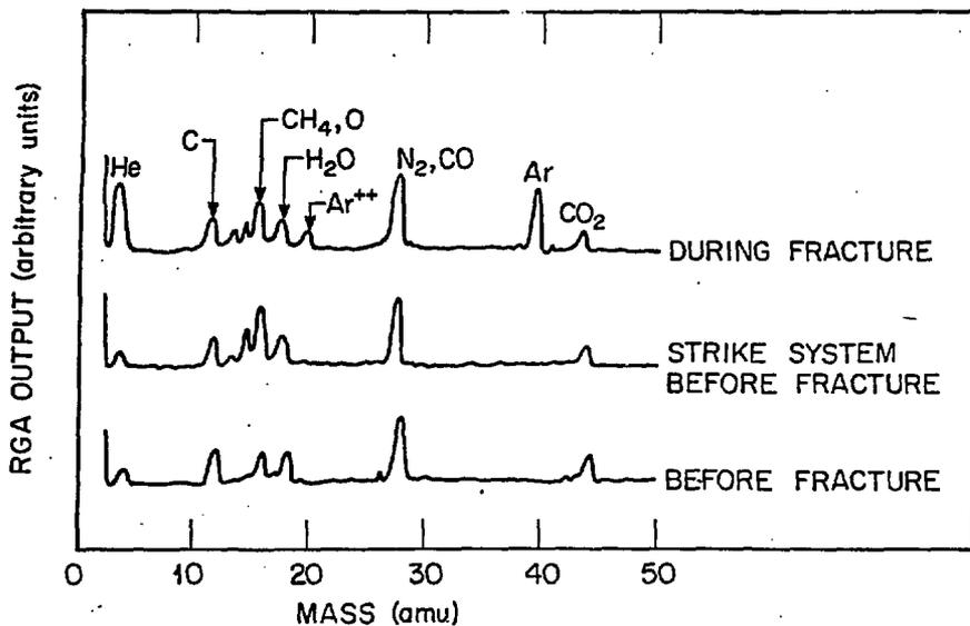
Fig. 12. Residual gas analyser (RGA) spectrum taken during fracture of the  $\alpha$ -SiC tubes in Figs. 10 and 11. The bottom curve shows the RGA spectrum before fracture, and the middle spectrum illustrates the effect of striking the system without fracturing the specimen.
