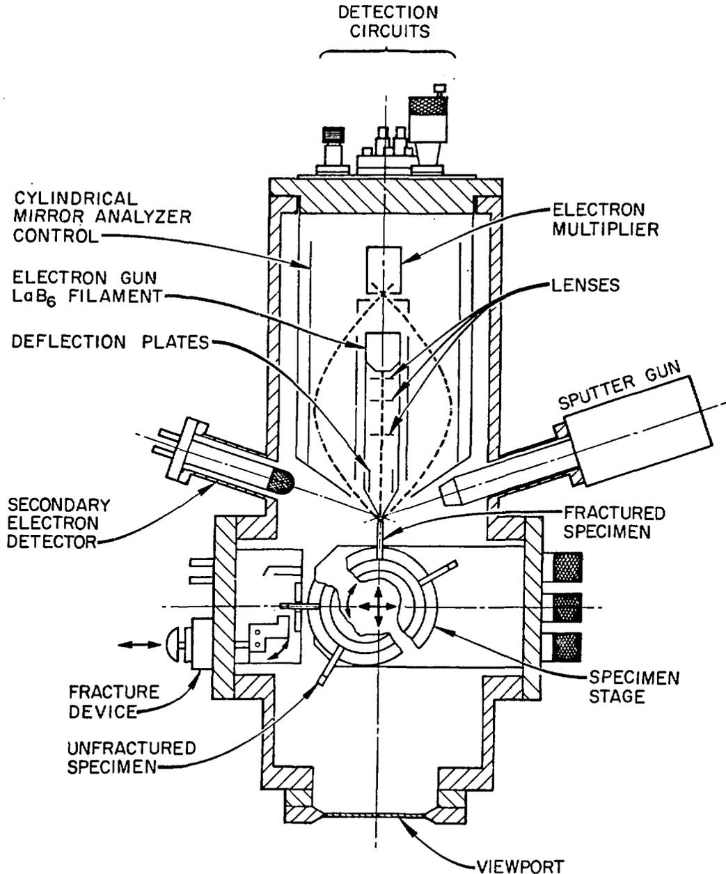
Fig. 7. Schematic view of a conventional AES analysis chamber incorporating a cylindrical mirror analyser (CMA) with a coaxial scanning electron gun. Curved dashed lines show the electron trajectory through the CMA.
