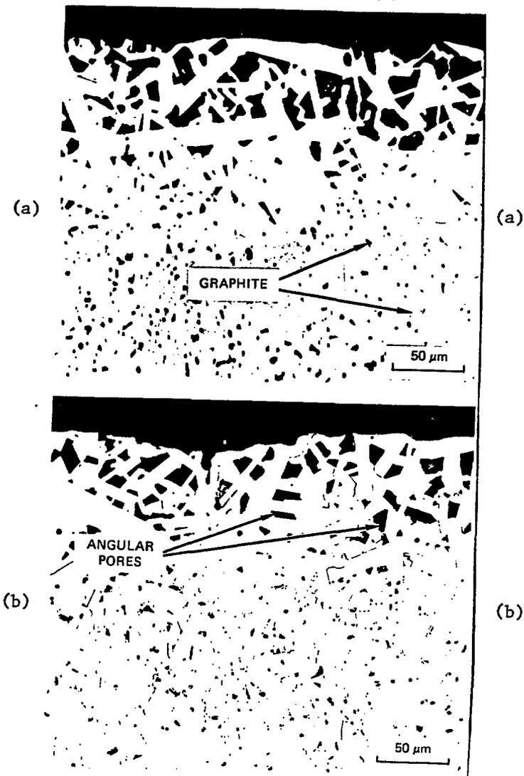
Fig. 10. Optical micrograph of sintered  $\alpha$ -SiC tubes exposed to a steel soaking pit environment.
