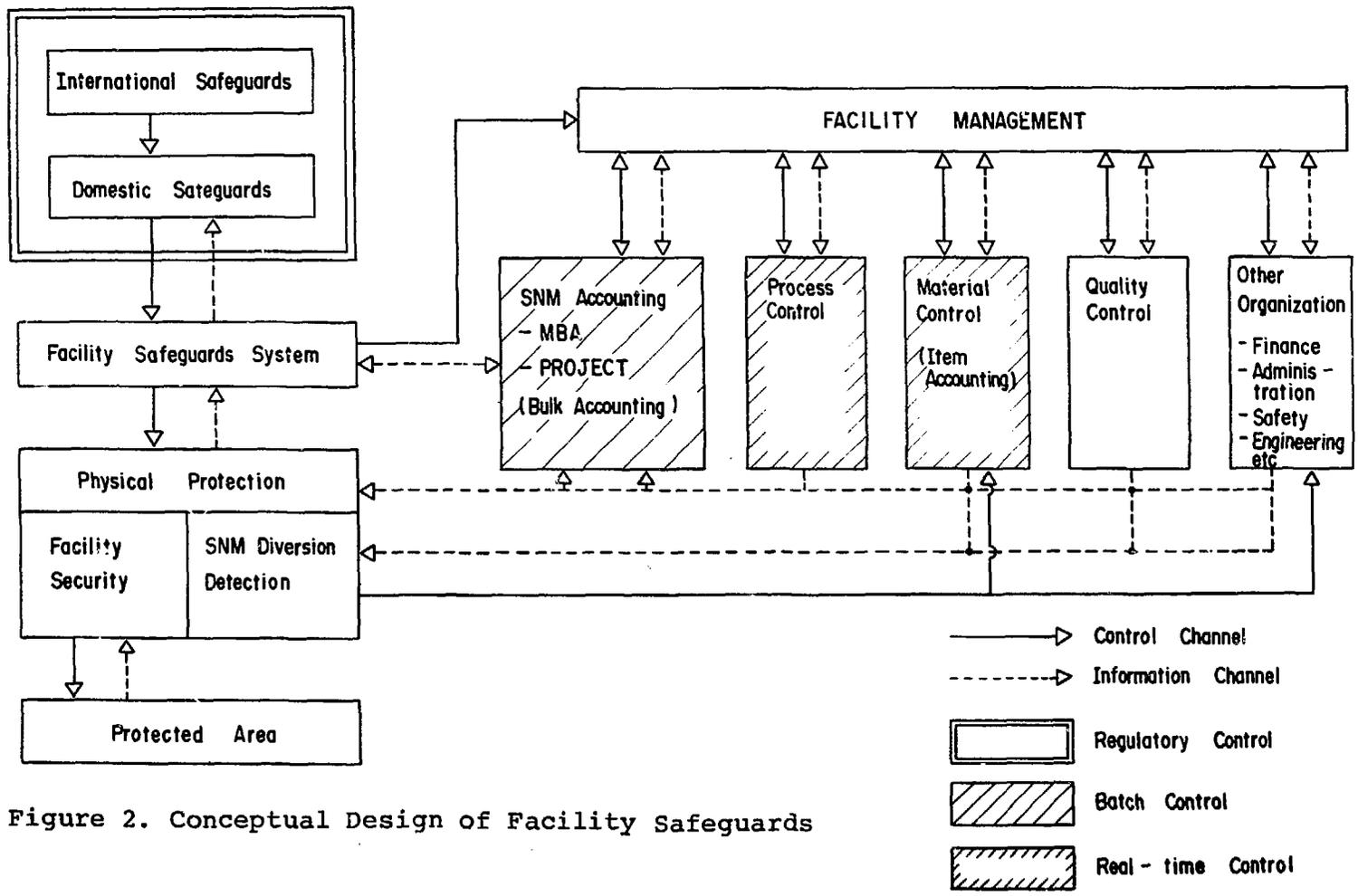
Figure 2. Conceptual Design of Facility Safeguards
