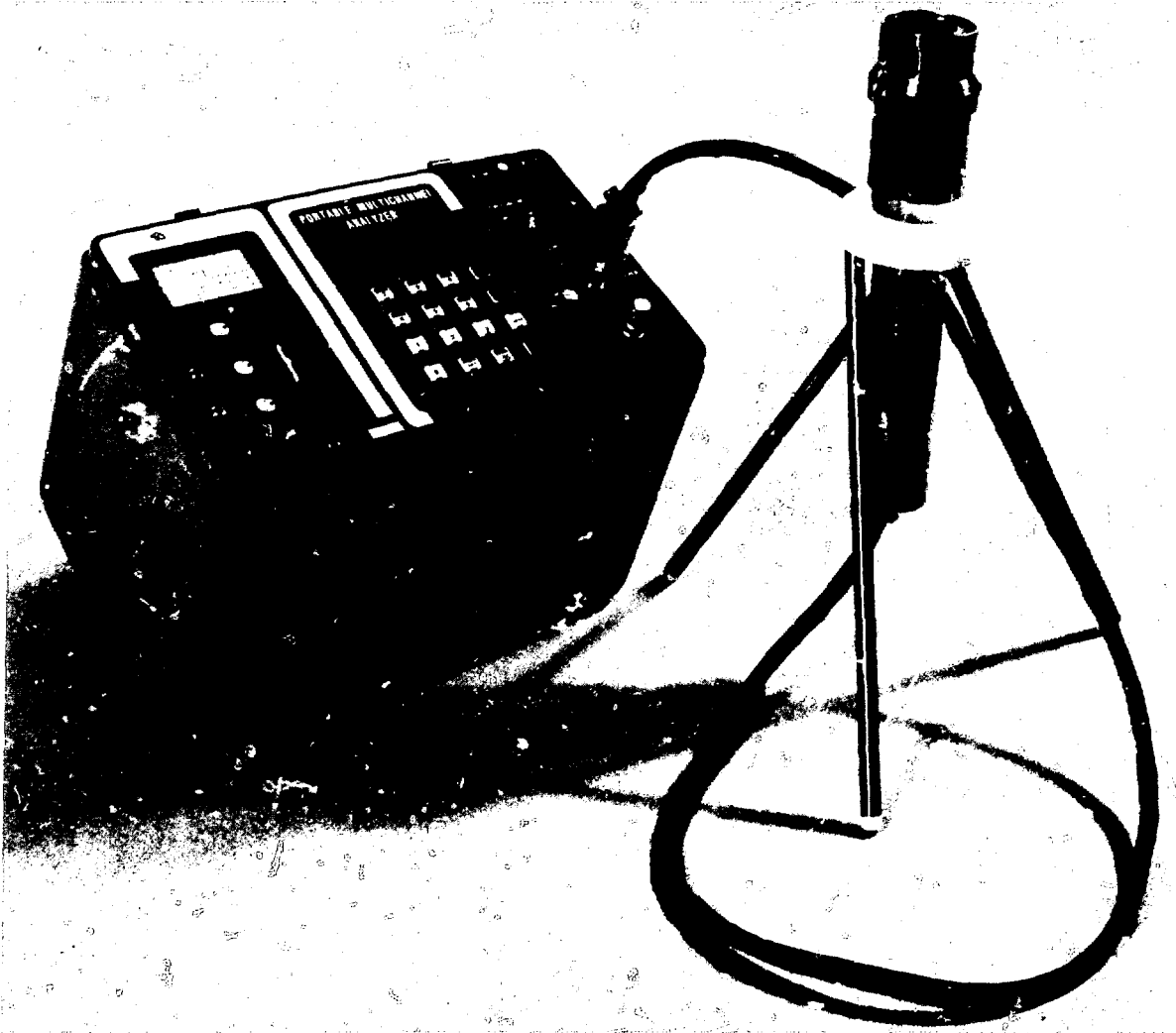
The Los Alamos Portable Multichannel Analyzer, along with the NaI detector in the configuration appropriate for enrichment measurements. The analyzer is battery powered and contains sufficient measurement and analysis software to direct and carry out a complete enrichment measurement.
