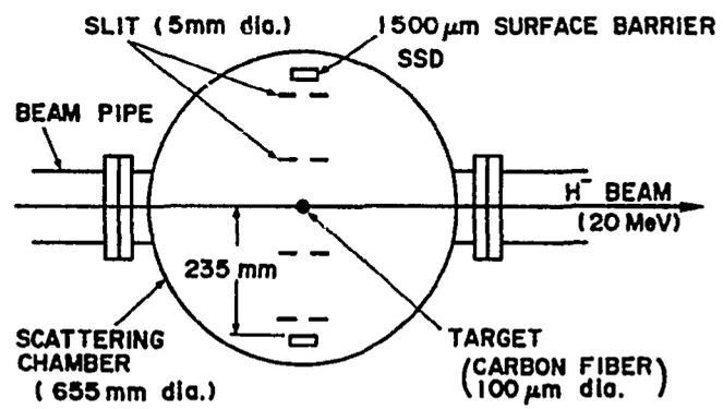
Fig. 3 Schematic of the 20 MeV polarimeter.
