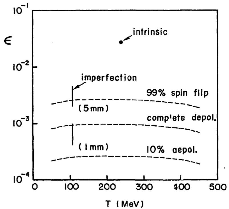
Fig. 1 Depolarizing resonances in the booster.
