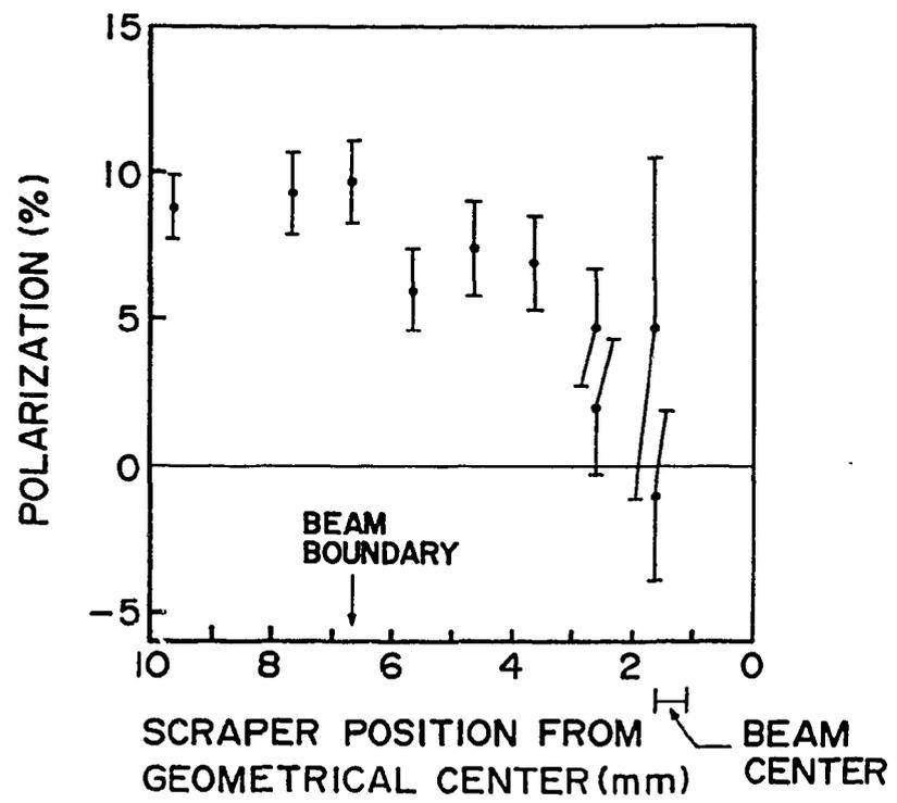
Fig. 8 Polarization vs. the vertical beam size in the booster.
