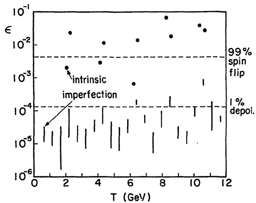
Fig. 2 Depolarizing resonances in the main ring.
