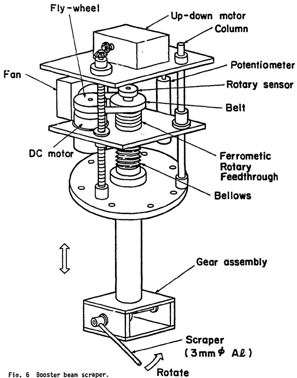
Fig. 6 Booster beam scraper.
