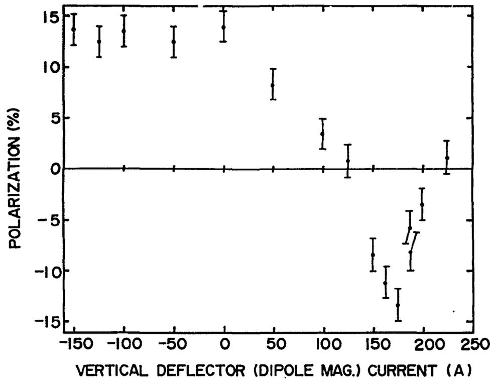
Fig. 9 Polarization vs. the excitation current of the vertical deflector.
