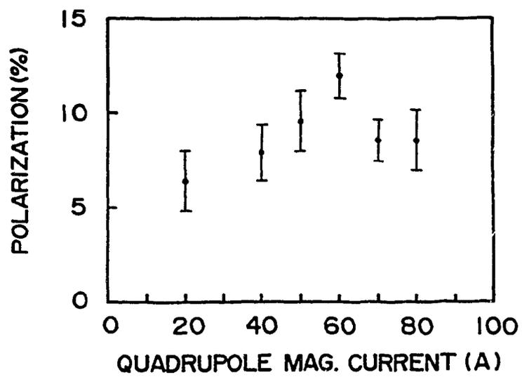
Fig. 10 Polarization vs. the excitation current of the correction quadrupole magnet.
