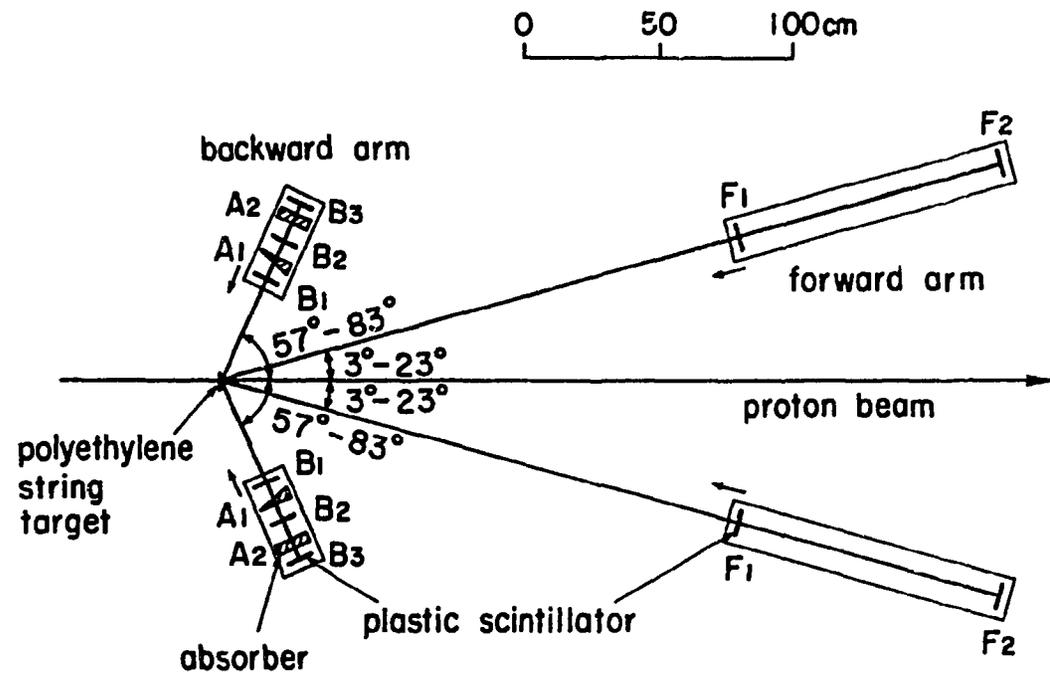
Fig. 4 Schematic of the main ring polarimeter.
