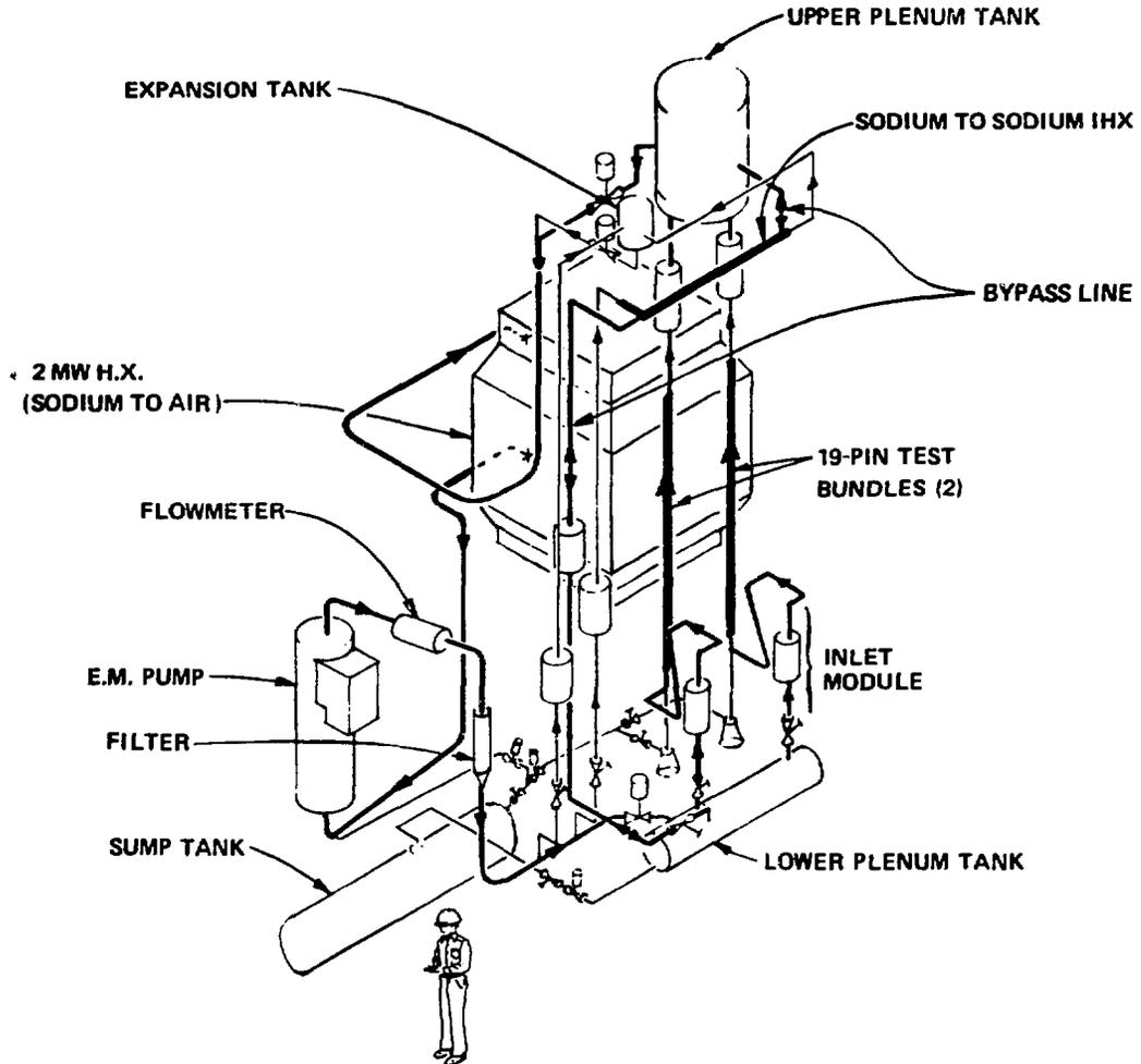
Fig. 1. THORS-SHRS facility isometric flow sheet.
