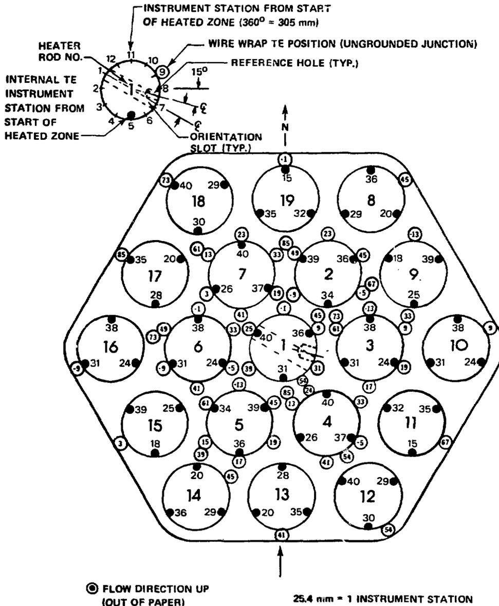
Fig. 3. THORS-SHRS Assembly 1 bundle thermocouple layout.
