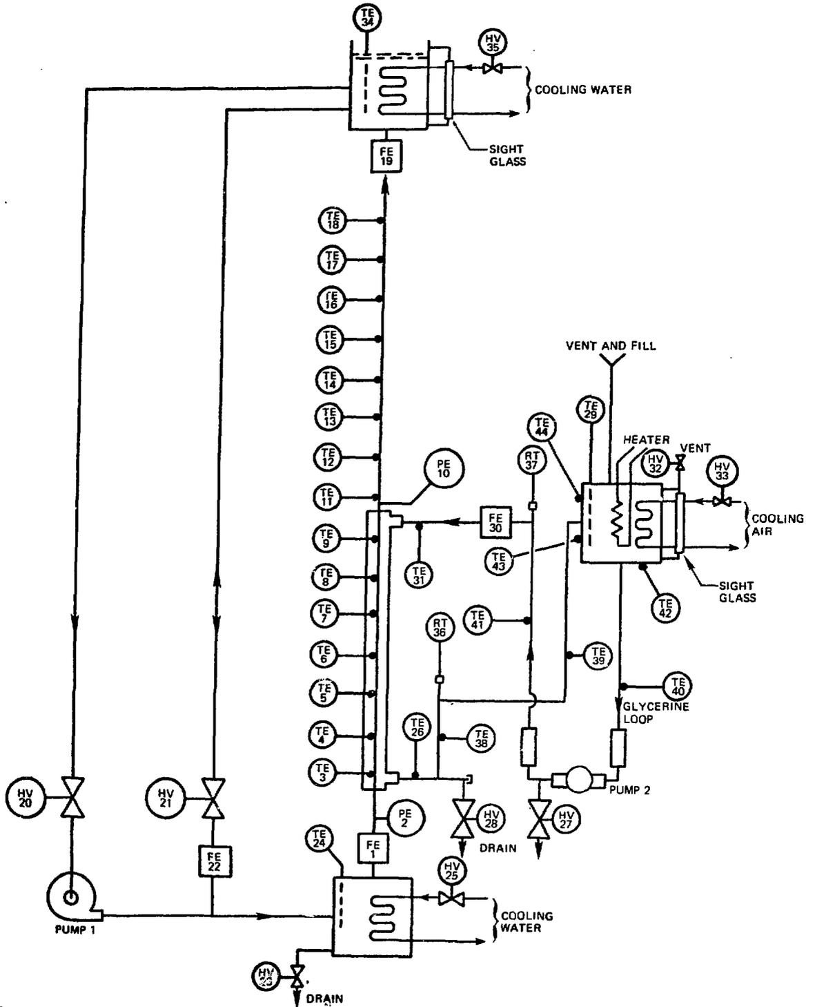
Fig. 8. SBFV loop design and instrumentation.
