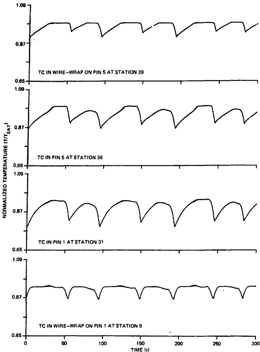
Fig. 5. Bundle temperatures during THORS-SHRS Assembly 1 Test 231A (see Fig. 3 for thermocouple locations).
