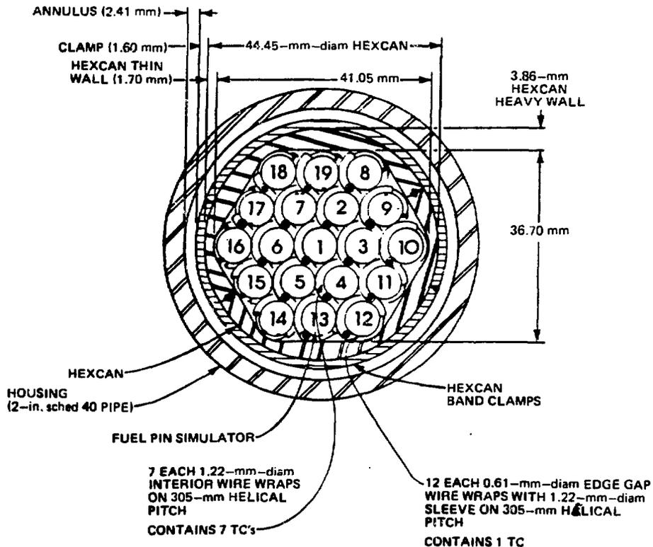
Fig. 2. Longitudinal and cross-sectional views of THORS-SHRS Assembly 1 bundle.
