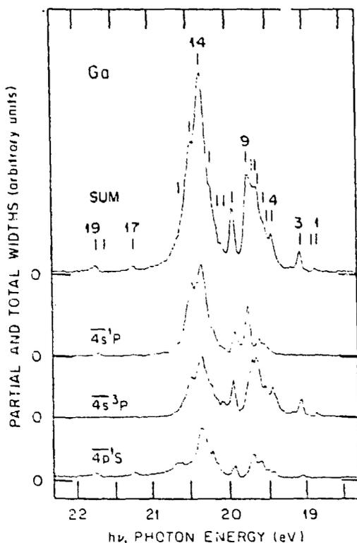
Fig. 3 The partial widths of the decay channels and the total width of the  $3d+4p$  resonance in atomic gallium as recorded in the CIS mode of operation. The top spectrum is virtually identical with the absorption spectrum.
