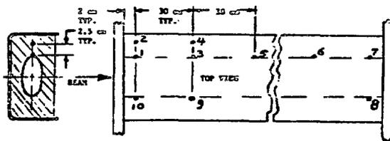
Fig. 2 - Thermocouple locations in the absorber block.
