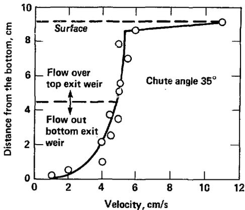
Fig. 5 Velocity profile of two-layered sand flow down a chute inclined at 35°. The entrance weir was 6 cm high. Flow rate, measured separately in two exit containers, was 1510 cm<sup>3</sup>/s, with 60% of the flow passing over the top exit weir.
