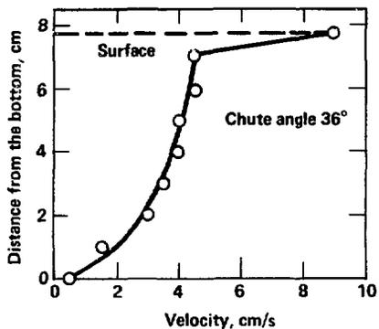
Fig. 4 Velocity profile of two-layered sand flow down a chute inclined at 36°. The entrance weir is 4 cm high. Flow rate, measured in a single exit container, was 940 cm<sup>3</sup>/s.
