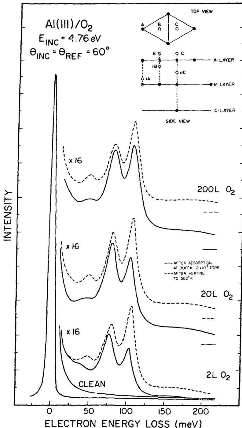
Figure 1 EELS spectra for 2, 20, and 200 L (1L =  $10^{-6}$  Torr sec) O<sub>2</sub> on Al(111) before and after annealing. The 80-meV peak corresponds to surface oxygen and the 105-meV peak corresponds to subsurface oxygen, and the 105 meV peak results from coupling of first and second Al layers through the subsurface oxygen. Inset: lattice model for the Al(111) surface showing possible positions for overlayer (B and C) and underlayer (tB, tA and Oc) oxygen atoms.
