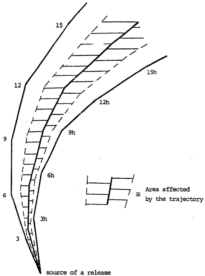
Fig.1 Affected area in the TRADOS model is determined by three subsequent trajectories.
