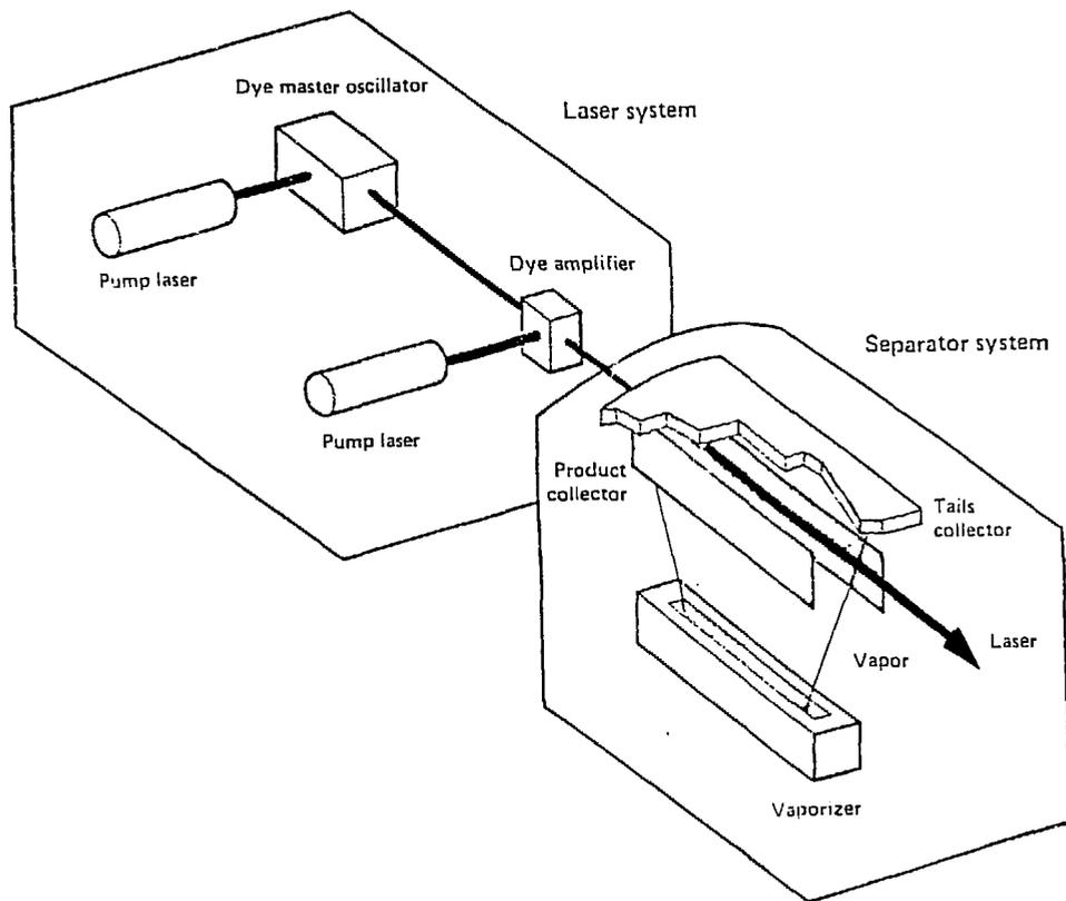
Figure 1. Atomic Vapor Laser Isotope Separation Diagram.
