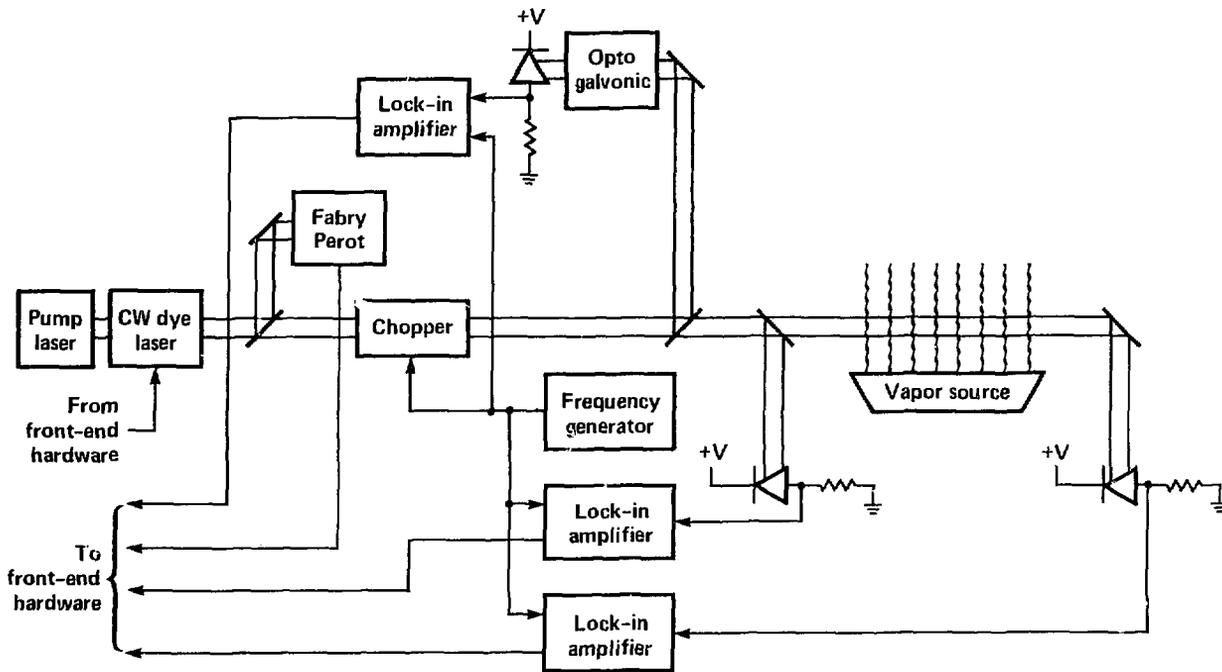
Fig. 8. Absorption spectroscopy hardware configuration.
