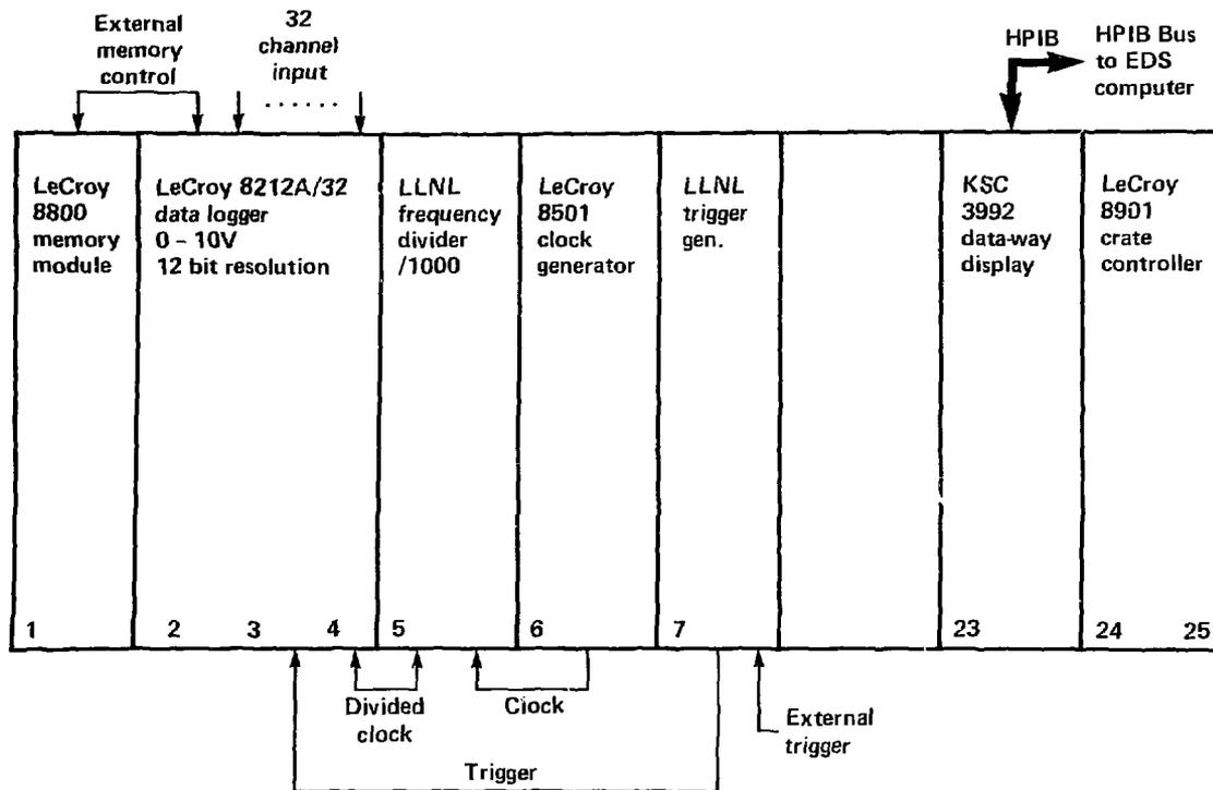
Fig. 6. Hardware configuration for process laser characterization.
