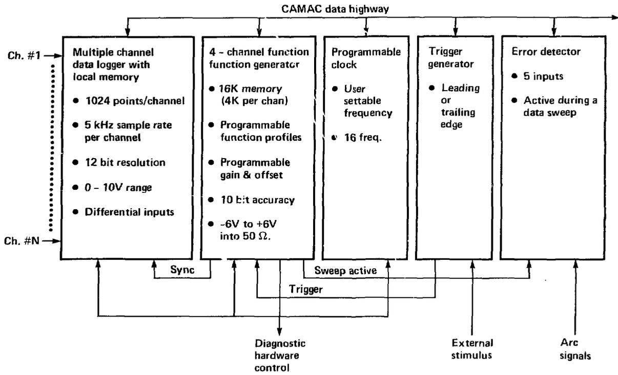
Fig. 3. CAMAC hardware configuration.
