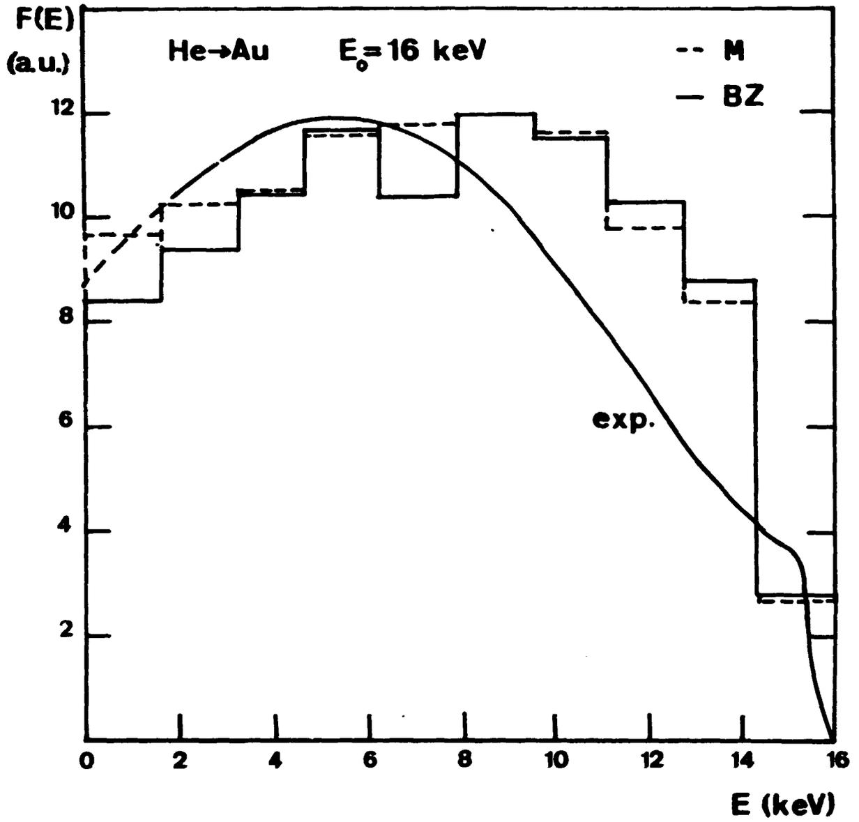
Fig.4: Energy distributions of helium backscattered from gold, discussed in Section 5. Solid curve, experimental result, from ref. [12]; dashed histogram: Molière simulation; solid histogram: Biersack-Ziegler simulation. Curve and histograms are normalized at their maximum.
