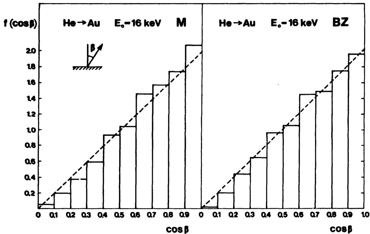
Fig.3: Angular distributions of helium backscattered from gold, discussed in Section 5. The independent variable is the cosine of the exit angle  $\beta$ .
