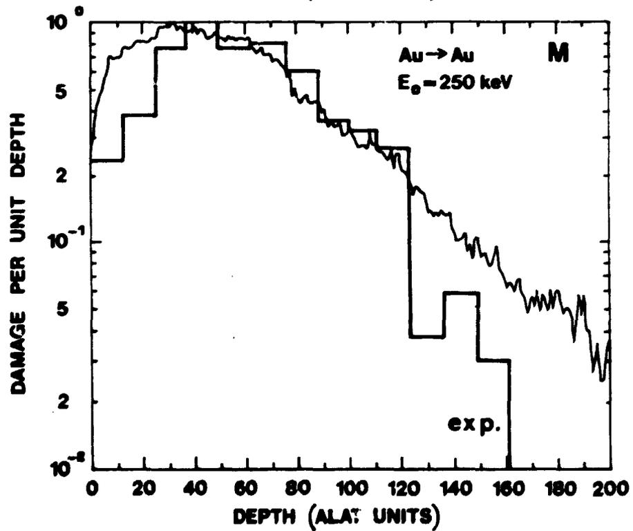
Fig.2: Distribution of vacancies per unit depth versus depth (in units of the lattice constant) for the self-irradiation of gold discussed in Section 4. BZ : damage profile calculated by means of the Biersack-Ziegler potential. M: the same profile calculated by means of the Molière potential, with modified screening length. EXP: experimental distribution of defect clusters from ref. [10]. Experimental and calculated profiles are normalized at their maximum.
