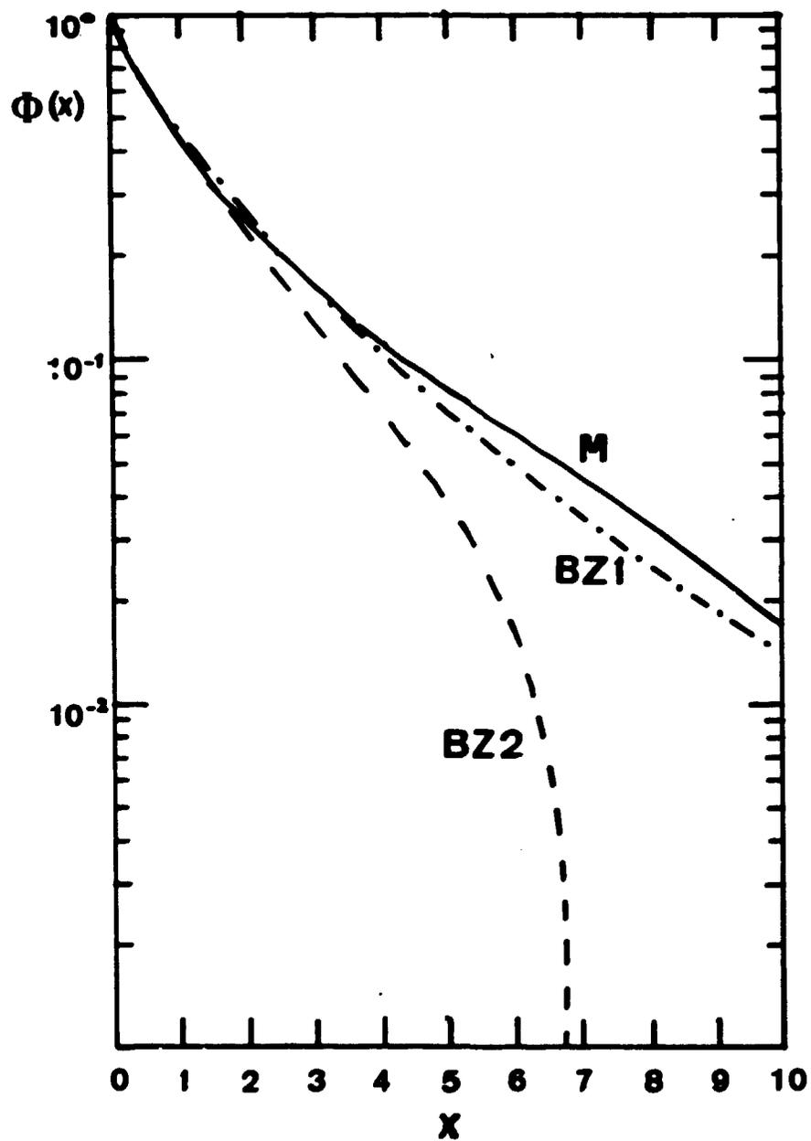
Fig.1: Screening functions versus interatomic distance  $x$ , in units of the Firsov length (formula (3)): M : Molière; BZ(Au-Au) (BZ1): Biersack-Ziegler, for gold-gold interactions; BZ(D-C): Biersack-Ziegler, for deuterium-carbon interactions (BZ2).
