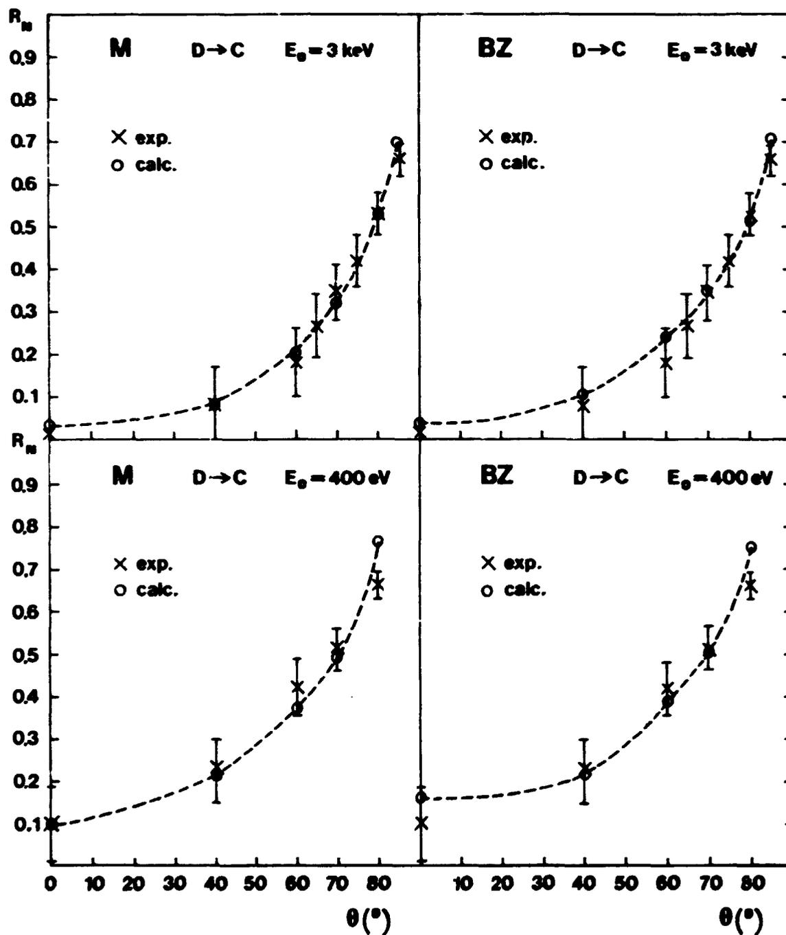
Fig.5: Particle reflection coefficient,  $R_N$ , for deuterium impinging on graphite, as a function of the angle of incidence  $\theta$ ; M: Molière; BZ: Bierack-Ziegler; the experimental data are from ref. [14].
