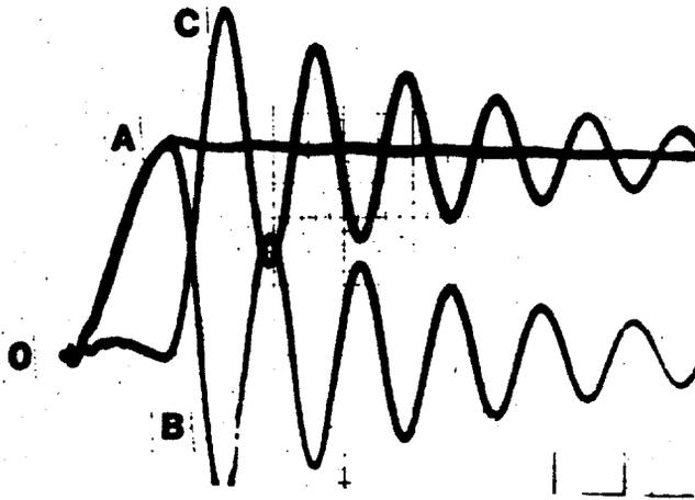
Figure 2. A) Magnet Current, B) Switch Current, C) Diode Current,  $V_c = 35$  kV, All 5 kA/div, 2  $\mu$ s/div
