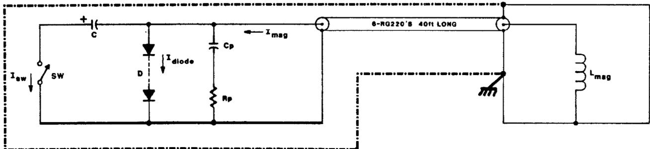
Figure 1. Simplified Pulse Power Circuit of Abort Pulser
