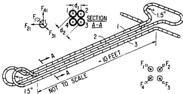
Fig. 13. Low Inductance HV Water Cooled Resistor Module
