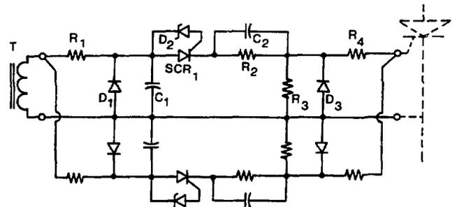
Fig. 9. Thyristor Pulse Shaping Network
