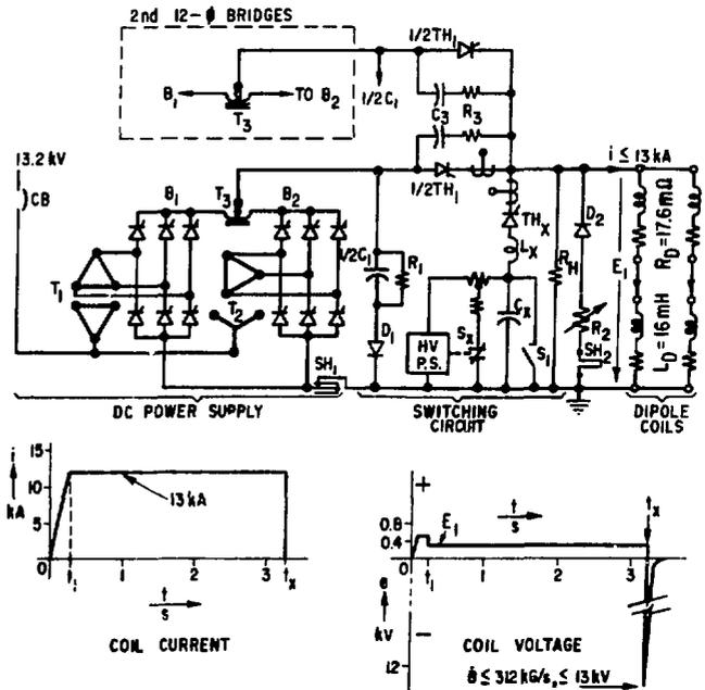
Fig. 3. Block Diagram of Dipole Power Supply
