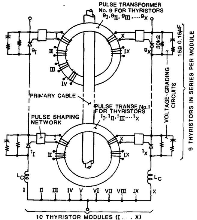
Fig. 8. Diagram of Thyristor Pulse Transformer Operation
