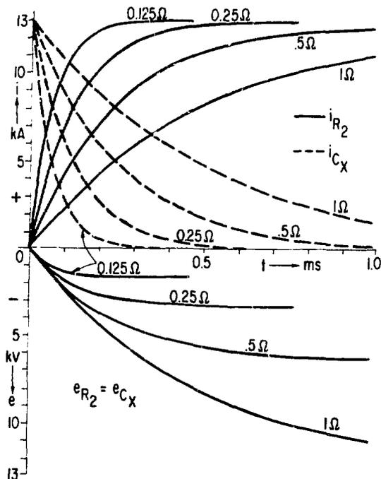
Fig. 5. Current and Voltage During Transfer of Current From Capacitor C<sub>x</sub> Into Crowbar Resistor R<sub>2</sub> for Various Values of R<sub>2</sub>.
