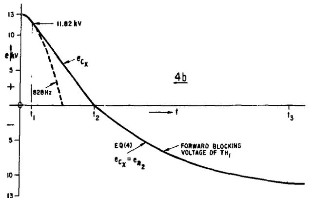
Fig. 4. Current and Voltage Waveforms of the Switching Circuit
