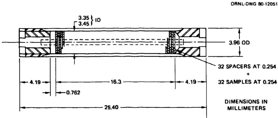
Fig. A.1. Transmission electron microscope (TEM) specimen holder.
