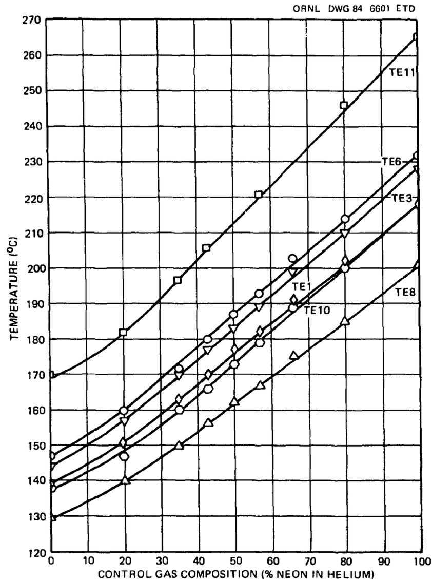
Fig. 3. Indicated temperatures for thermocouples (TE) vs percent neon in control gas region of the 200°C test region of MFE-6J prototype capsule.
