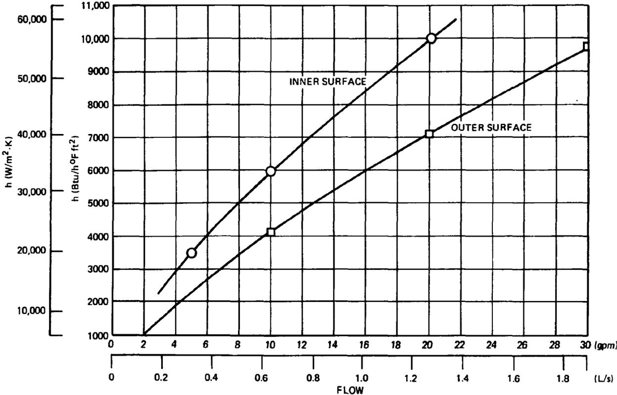
Fig. B.1. Surface heat transfer coefficients for 200°C region of capsule MFE-6J as a function of coolant flow rate.
