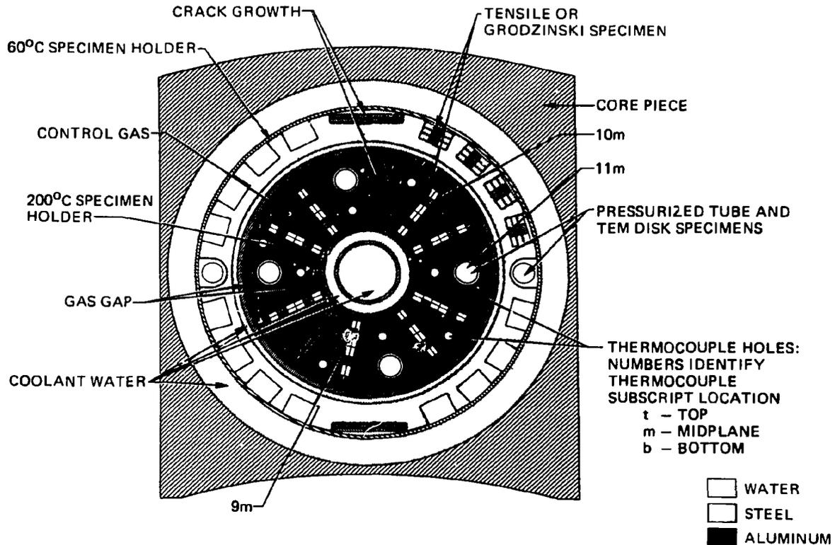
Fig. 1. Horizontal cross section through specimen region of irradiation capsule MFE-6J
