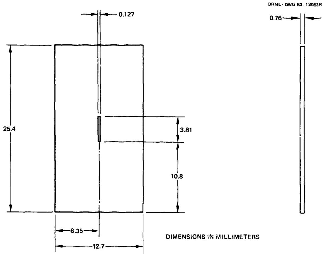
Fig. A.4. Crack-growth specimen. Tabs are welded along the 25.4-mm edge following irradiation.
