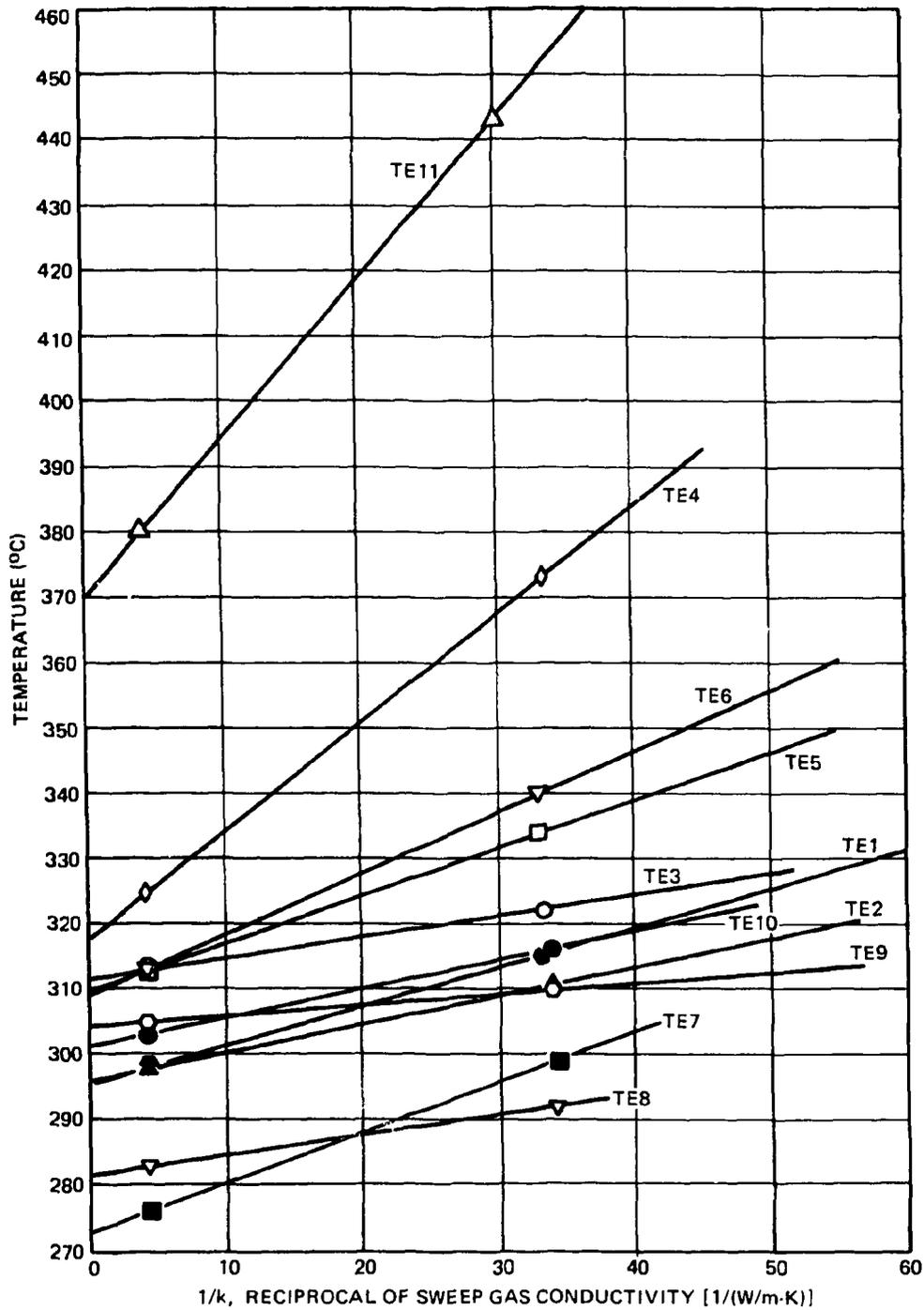
Fig. 5. Indicated temperatures in the 200°C test region of MFE-6J prototype capsule vs reciprocal of sweep gas conductivity with a control gas of 100% argon.
