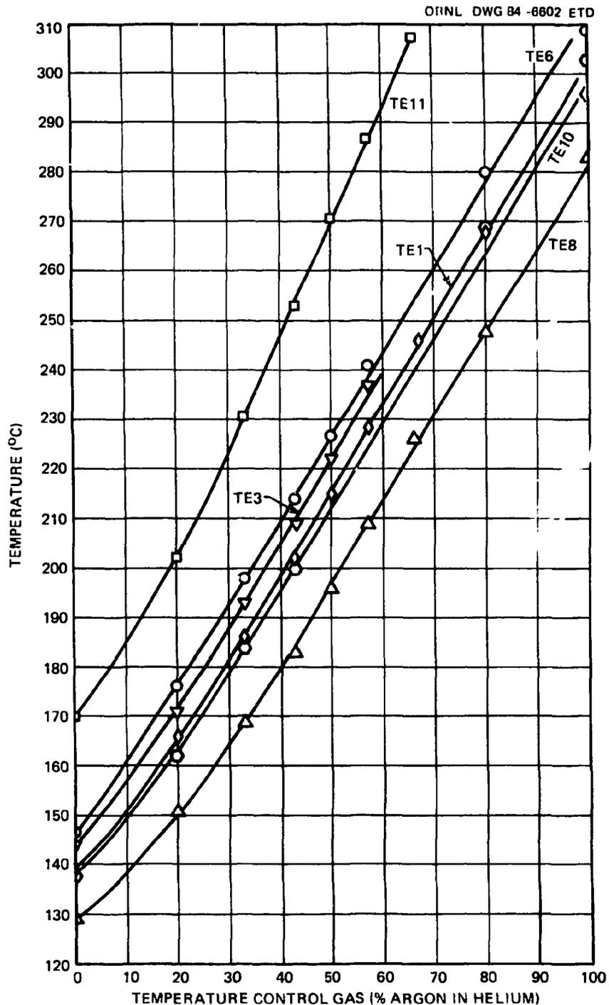
Fig. 4. Indicated temperature for thermocouples vs percent argon in control gas region of the 200°C test region of MFE-6J prototype capsule.
