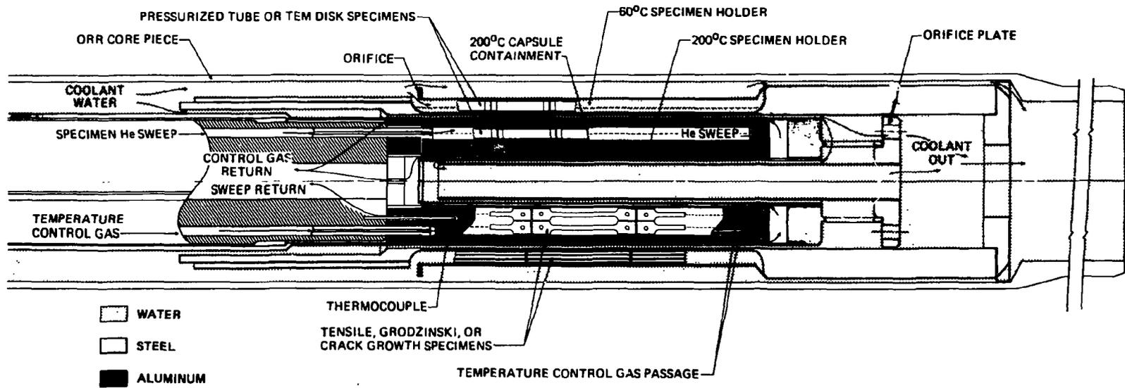
Fig. 2. Vertical cross section through in-core region of irradiation capsule MFE-6J.
