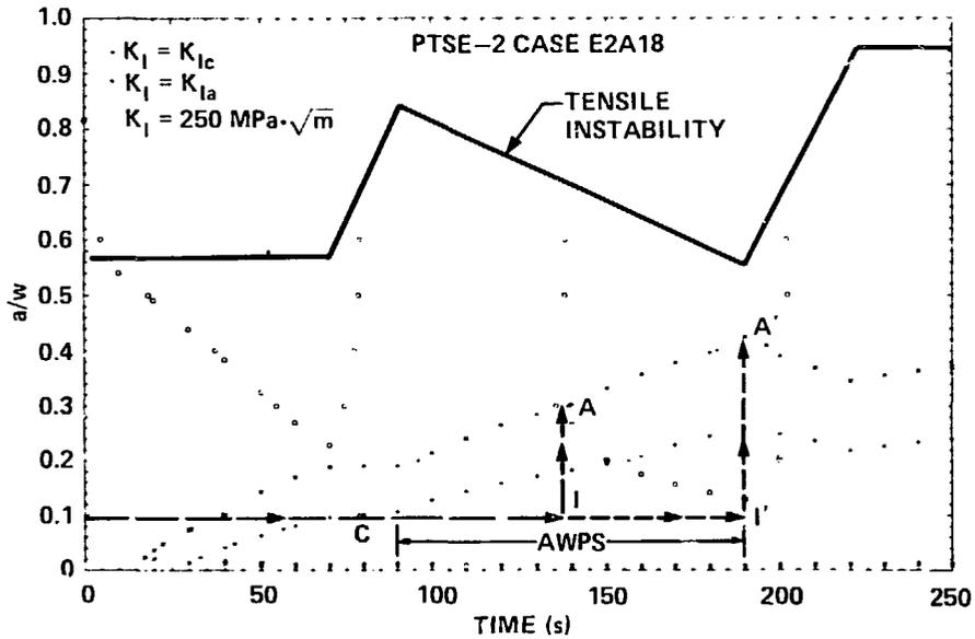
Fig. 11. Critical crack depth curves for crack initiation, arrest, and tensile instability. A crack initiating at point I would arrest when  $K_I$  is  $\sim 250 \text{ MPa}\cdot\sqrt{\text{m}}$ . This  $K_I$  value may be necessary to induce a tearing instability.  $a/w$  = ratio of crack depth to wall thickness.
