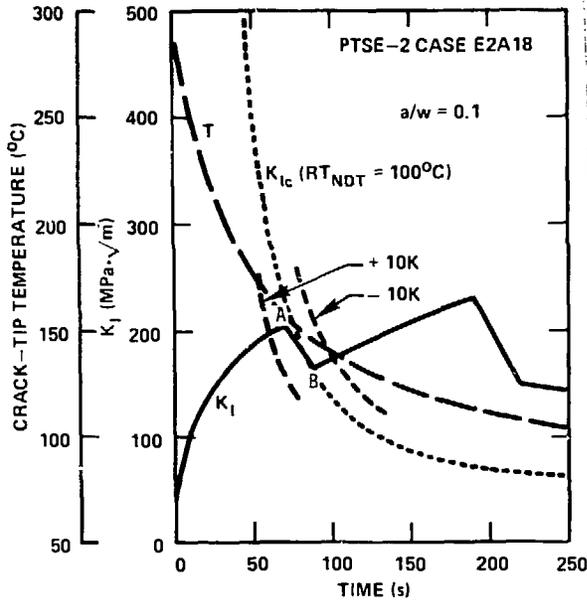
Fig. 7. Effect of uncertainty in  $K_{Ic}$  on the timing of a warm-prestressing phase. Curve segments marked  $\pm 10K$  are the  $K_{Ic}$  loci for  $RT_{NDT}$  10K higher and lower, respectively, than the nominal value  $100^{\circ}C$ .
