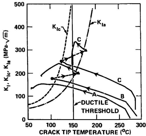
Fig. 3.  $K_I$ -temperature trajectory of the crack tip in the three PTSE-1 transients.
