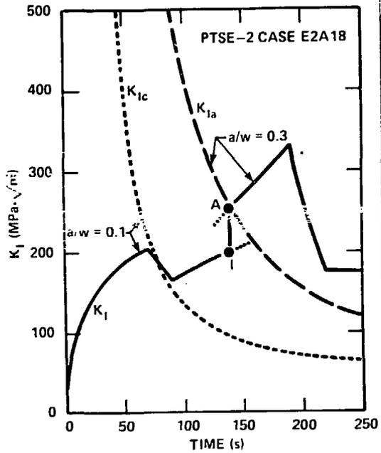
Fig. 9.  $K_I$ ,  $K_{Ic}$ , and  $K_{Ia}$  vs time for illustrative PTSE-2 transient in which it is presumed that the crack will propagate at point I during simple anti-warm prestressing. In this case the crack arrests at point A.
