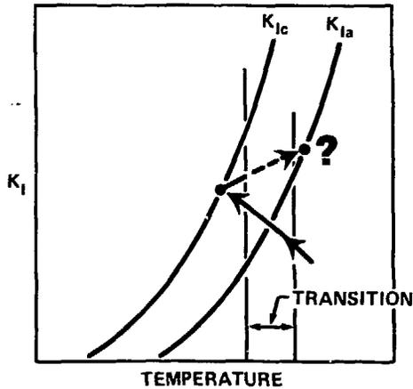
Fig. 8. Illustration of the temperature range in which the mode of fracture in a well-restrained structure is unknown.
