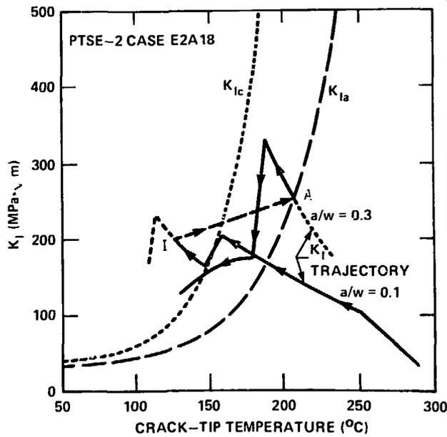
Fig. 10.  $K_I$ -temperature trajectory for the transient of Figs. 6, 7, and 9. This shows that, if the initial crack does not propagate,  $K_I$  will eventually become  $\sim 3$  times  $K_{Ic}$ .
