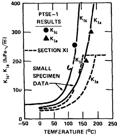
Fig. 5. Fracture toughness values derived from PTSE-1 data compared with pretest expectations and values prescribed by Section XI of the ASME Boiler and Pressure Vessel Code.
