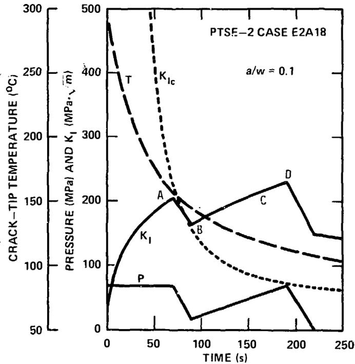
Fig. 6. Pressure, crack-tip temperature,  $K_I$ , and  $K_{Ic}$  transients for  $a/w = 0.1$  from a preliminary analysis of PTSE-2 based on speculative properties.
