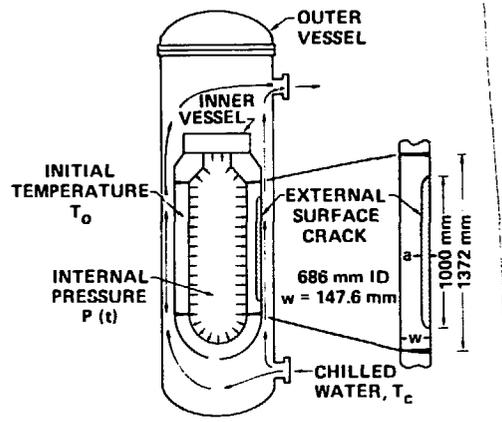
Fig. 1. Schematic view of pressurized-thermal-shock vessel inside shroud. Dimensions shown are for the PTSE-1 vessel.
