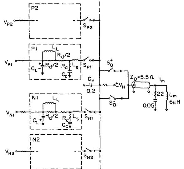
Fig. 4 The bipolar n-pulse modulator circuit
