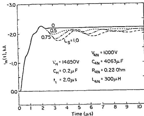
Fig. 6 The effect of stray inductance  $L_s$  on the front end of the pulse
