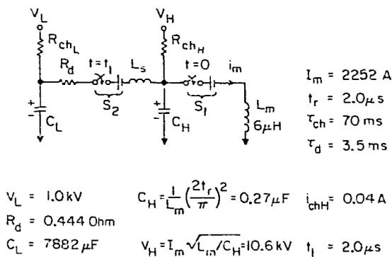
Fig. 3 A two-section single pulse circuit
