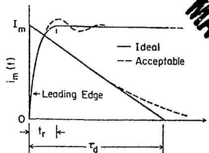
Fig. 2 Required pulse waveform
