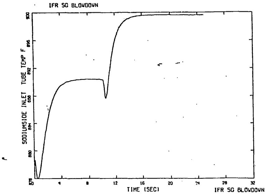
Figure 11. Sodium Side Tube Temperature Inlet Nozzle
