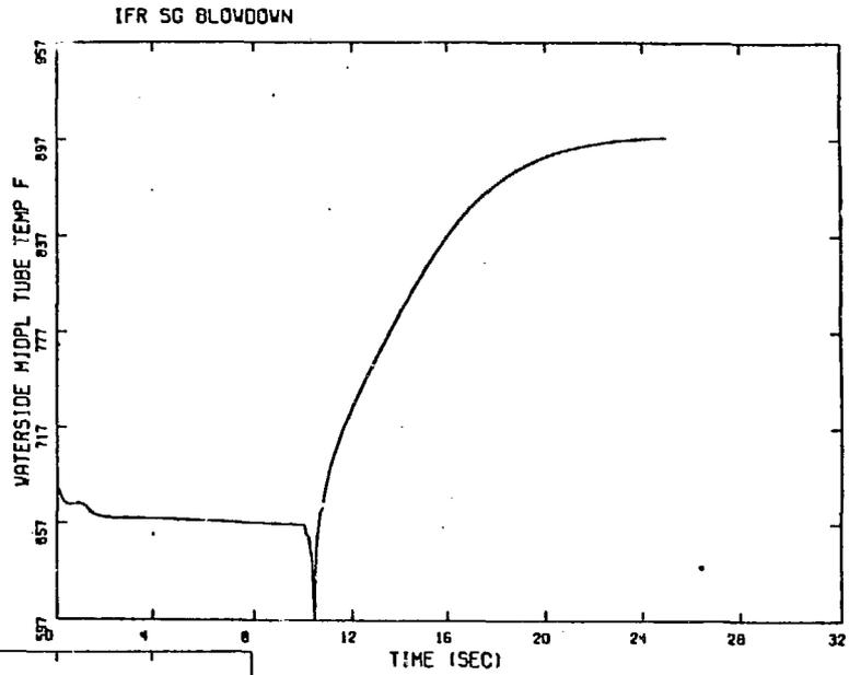
Figure 15. Water Side Tube Temperature Midplane
