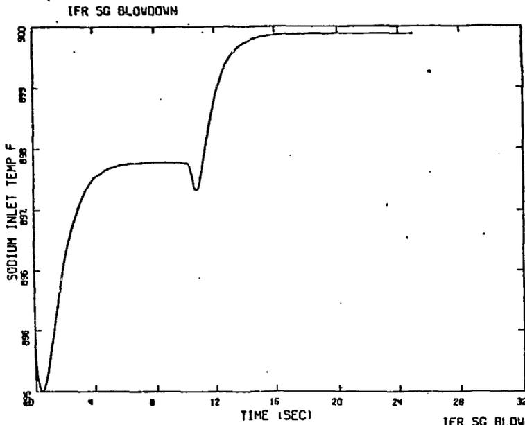
Figure 8. Sodium Temperature Inlet Nozzle
