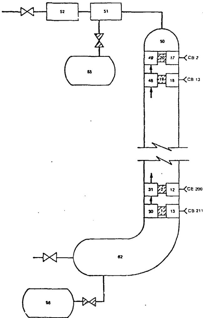
Figure 4. RETRAN Stand-alone Steam Generator Model
