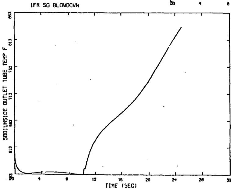
Figure 13. Sodium Side Tube Temperature Outlet Nozzle
