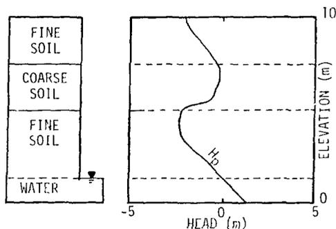
Figure 4. Layered soil column during steady flow conditions.
