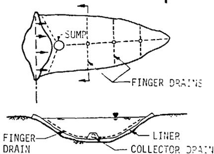
Figure 6. Interior drainage system utilizing finger drains.
