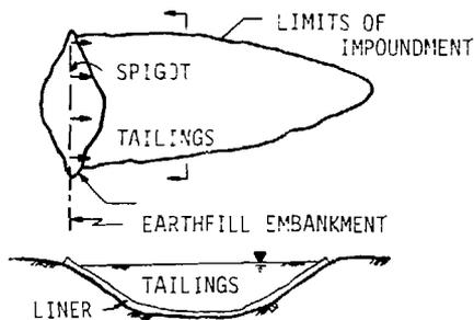
Figure 5. Typical existing impoundment without internal drainage.
