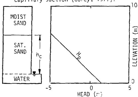
Figure 3. Drained sand column under equilibrium conditions.
