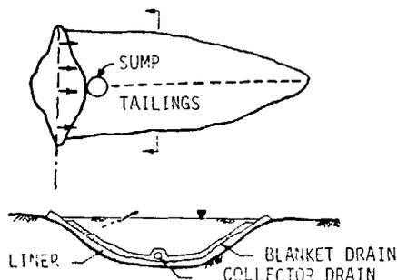
Figure 7. Interior drainage utilizing a blanket drain.
