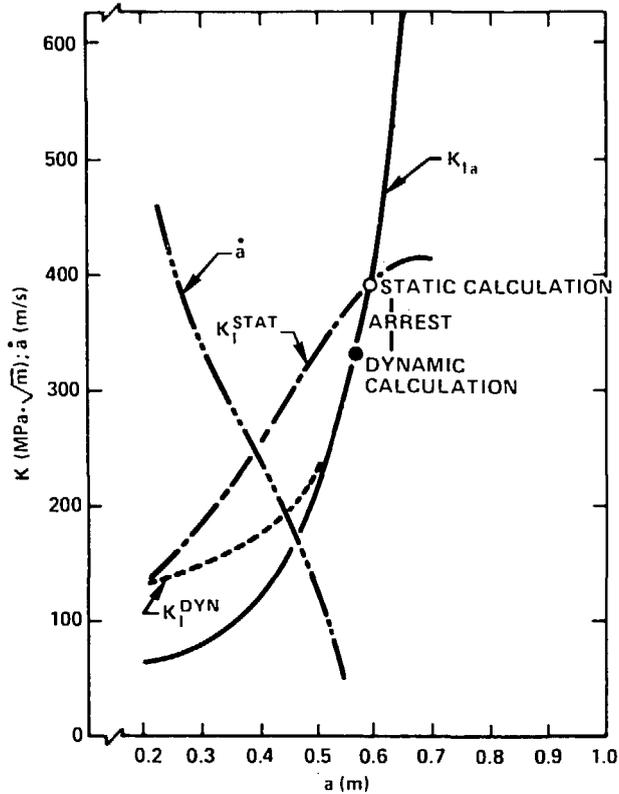
Fig. 3. Schematic of dynamic effects during a crack run-arrest event in a wide-plate specimen where the crack-tip temperature increases with crack depth.
