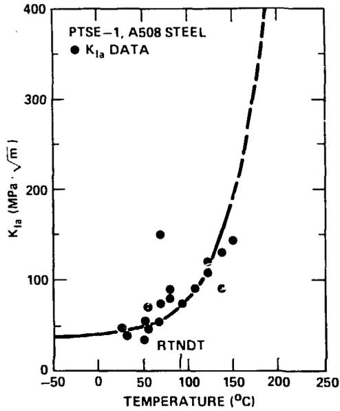
Fig. 5. Crack-arrest data for HSST PTSE-1 material from tests at Battelle Columbus Laboratories using laboratory-size specimens.
