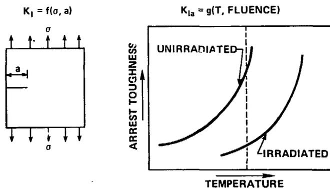
Fig. 2. Schematic illustration that crack arrest occurs when the driving force ( $K_I$ ) reaches a critical toughness value ( $K_{Ia}$ ) which is dependent on temperature and irradiation exposure.
