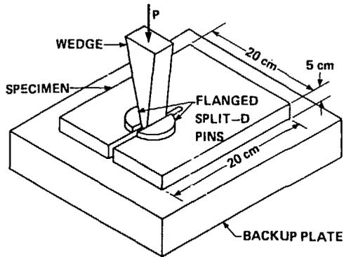
Fig. 6. Schematic of side-wedge-loaded compact specimen used in laboratory crack-arrest tests.
