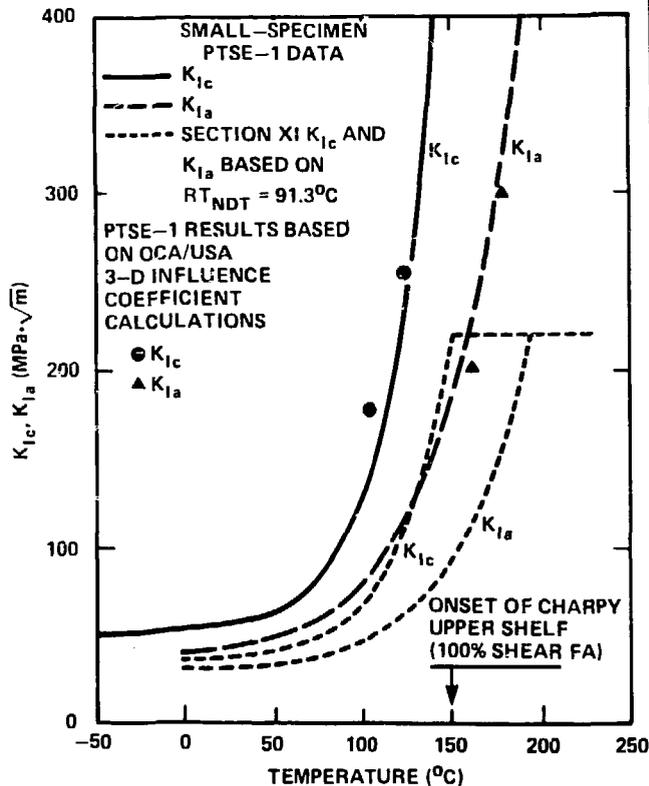
Fig. 8. Initiation and arrest toughness data from the first HSST pressurized-thermal-shock experiment (PTSE-1).
