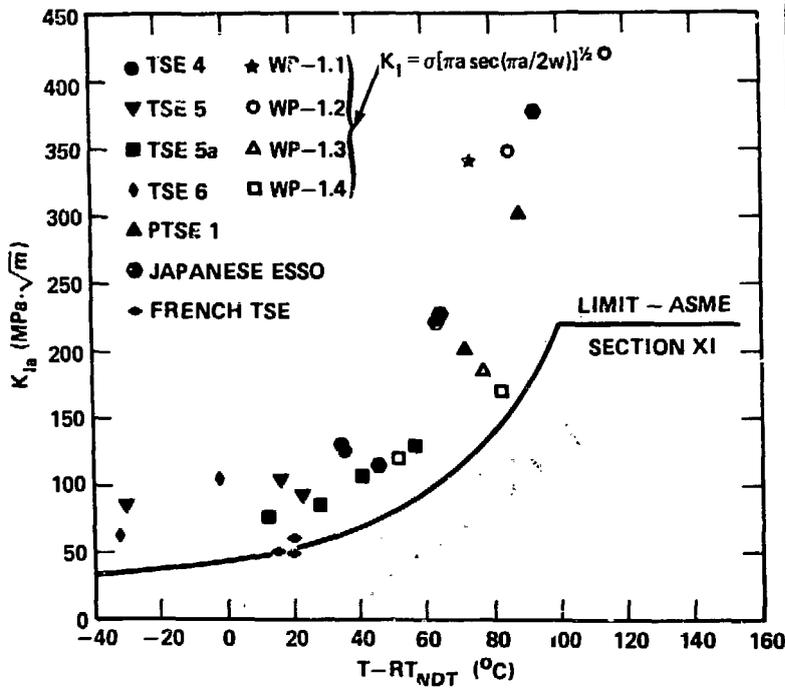
Fig. 10. Crack-arrest toughness data from large specimens show a consistent trend and extend above the ASME Section XI limit.
