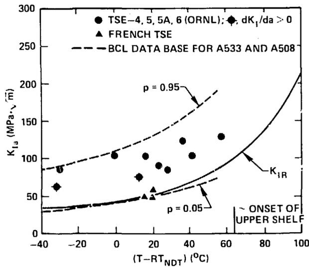
Fig. 7. Crack-arrest toughness data from thermal-shock experiments of thick-cylindrical specimens.
