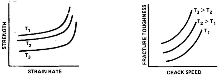
Fig. 4. Schematic illustration that strength and fracture toughness measures are temperature and rate dependent.
