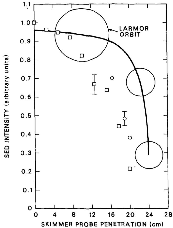
Fig. 3. Solid line: calculated radial profile of the fast-ion density; squares: measured radial profile of the fast-ion density; circles: calculated size of a 20-keV Larmor orbit as a function of radius (hydrogen beam).
