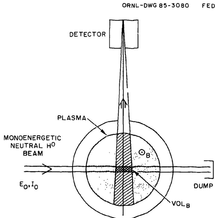
Fig. 2. Geometry of the fast-ion-decay method of determining the neutral density.
