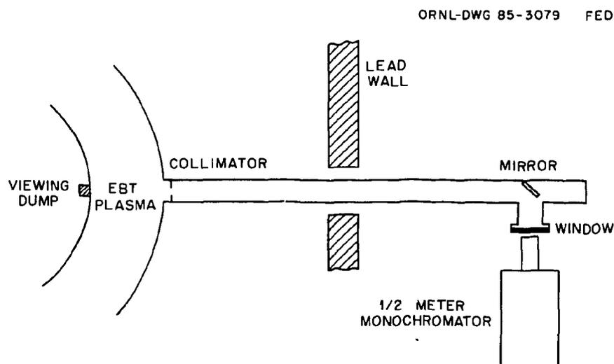
Fig. 1. Schematic of the optical system used in measuring both atomic and molecular emissions.
