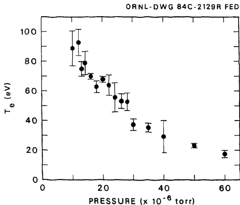
Fig. 4. The variation of the electron temperature with fill gas pressure at 100 kW of electron cyclotron heating (ECH) power. These data were obtained by Thomson scattering (Cobble 1985).
