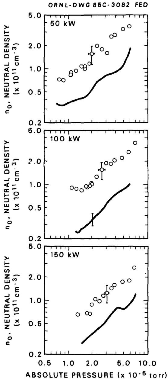
Fig. 6. The values of the neutral density for the conditions of figure 5.
