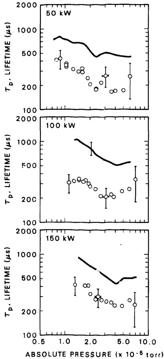
Fig. 5. The variation of the particle confinement time,  $\tau_p$ , determined by the two diagnostic techniques, as a function of fill gas pressure and at three input microwave powers: 50, 100, and 150 kW. The solid curve is from spectroscopy, and the circles are from fast-ion-decay measurements.
