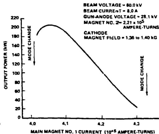
Figure 8. Peak Power Out vs Magnet No. 1.
