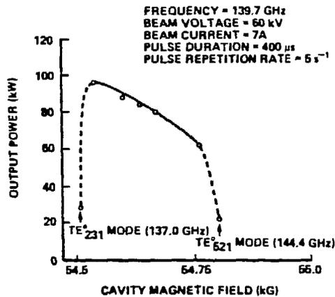
Figure 6. Output Power vs Cavity Magnetic Field for 140 GHz Gyrotron Operation in the  $TE_{031}$  Mode with a Beam Voltage of 60 kV and a Beam Current of 7 A.
