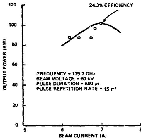
Figure 5. Output Power vs Beam Current for 140 GHz Gyrotron Operation in the  $TE_{031}$  Mode with a Beam Voltage of 60 kV and Optimized Magnetic Field.
