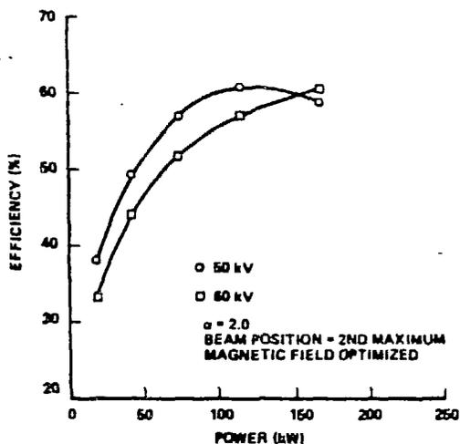
Figure 1. Efficiency vs Output Power for Simple TE<sub>031</sub> 140 GHz Cavity Designs.
