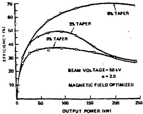
Figure 3. Calculated Efficiency vs Output Power for Different Magnetic Field Tapers for the 140 GHz  $TE_{021}/TE_{031}$  Cavity Design.
