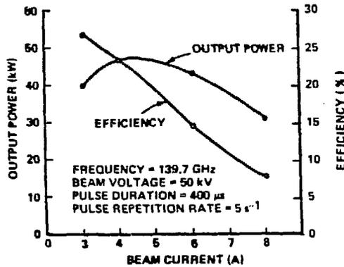
Figure 4. Output Power and Efficiency vs Beam Current for 140 GHz Gyrotron Operation in the  $TE_{031}$  Mode with a Beam Voltage of 50 kV.
