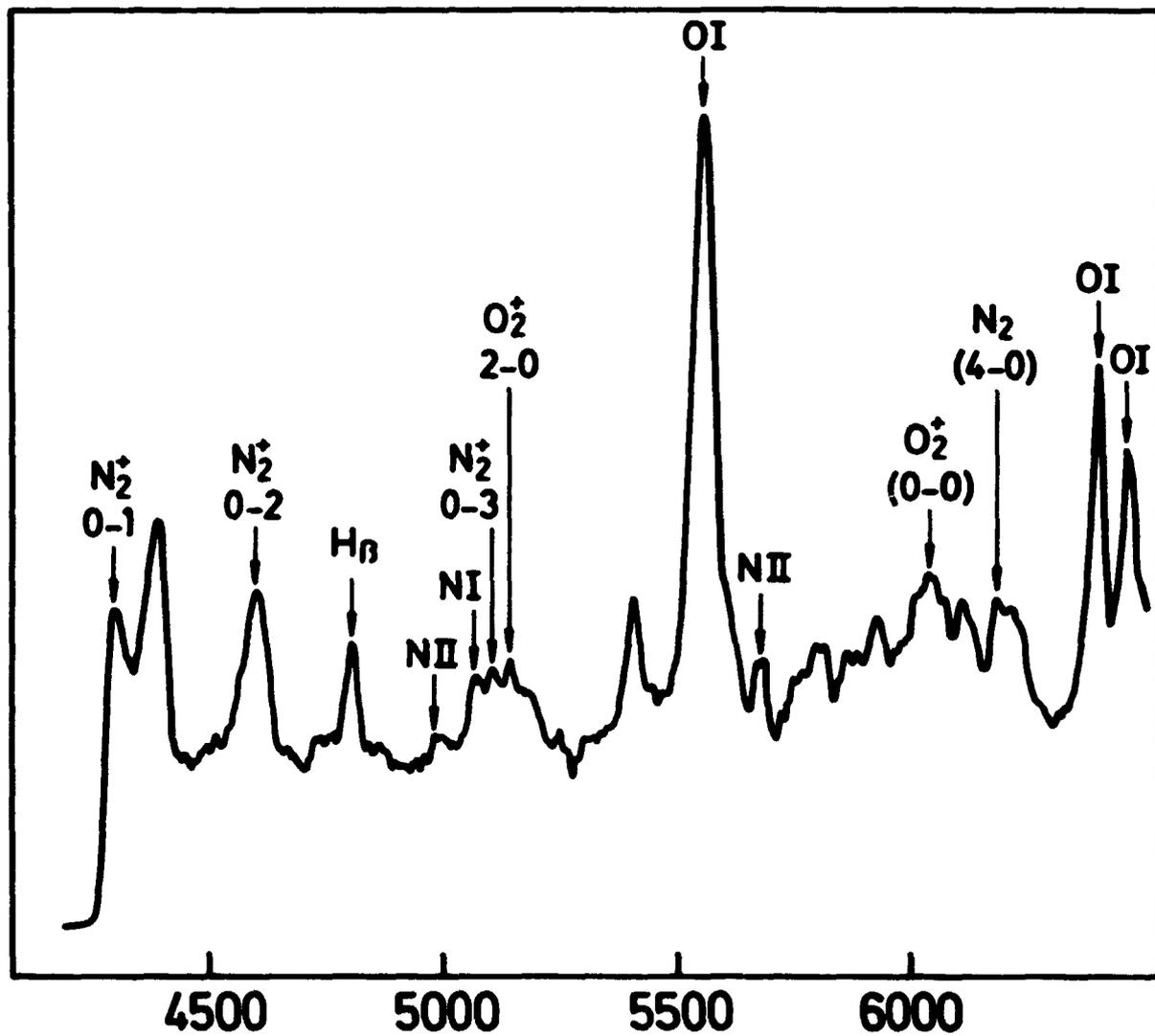
Fig. 1 Spectrogram of the observed spectral region 4200-6400 Å.
