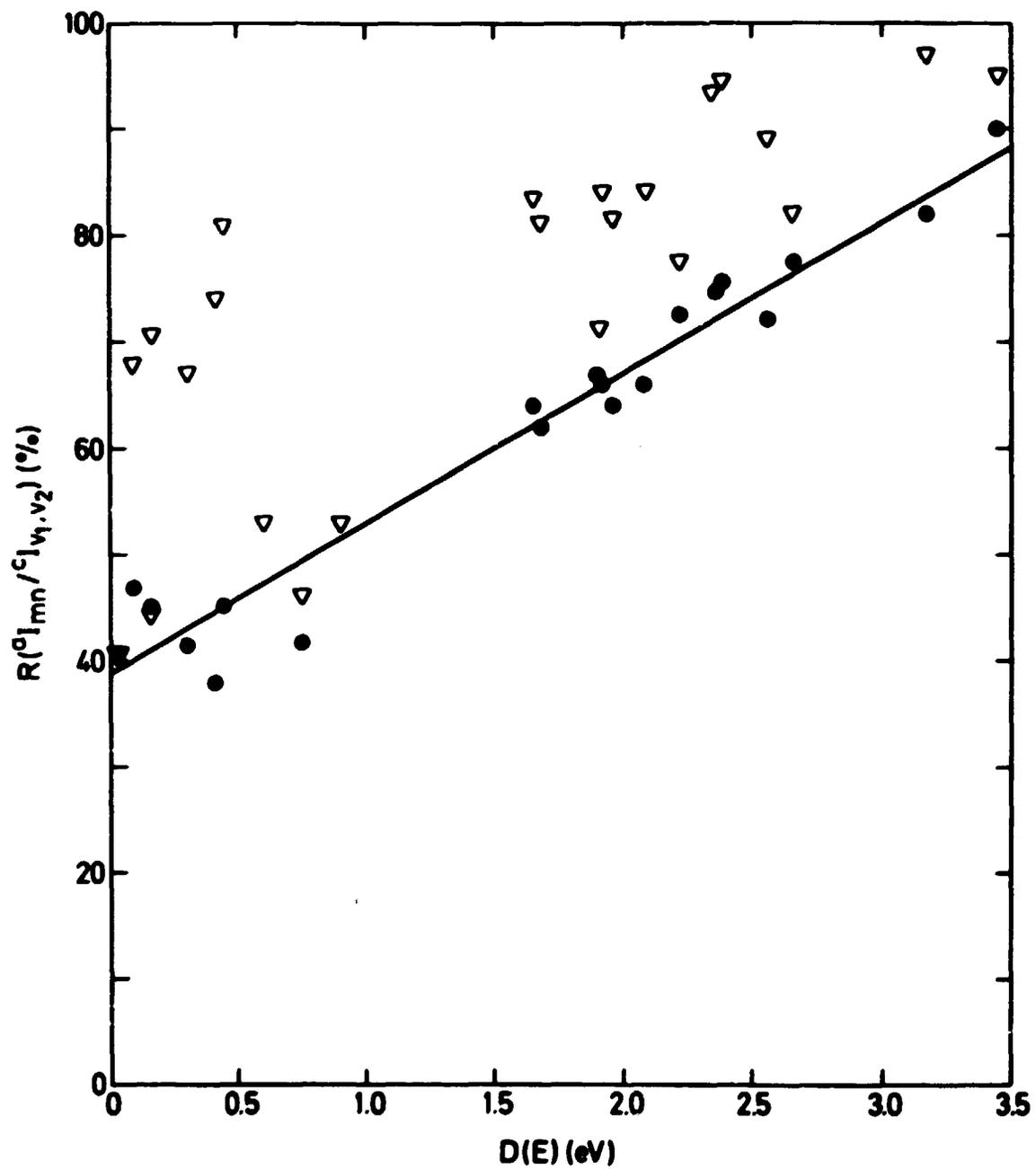
Fig. 2 RD-graph from auroral measurements of a whole night (8 hours). The triangular points are uncorrected and the filled circular points represent atomic transitions, which are  $\sigma$ -corrected.
