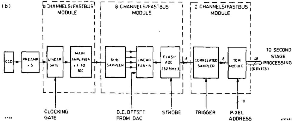
Fig. 3. (a) and (b) Vertex Detector Configuration and Electronics Channel Block Diagram.
