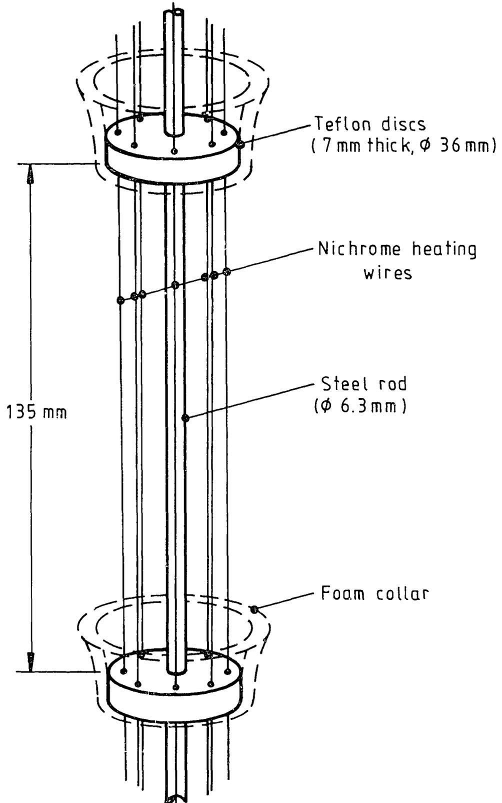
Figure 1 Section of the heat source probe.
