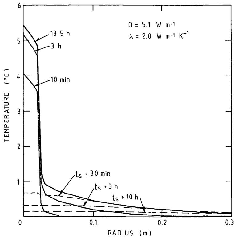
Figure 3 Radial temperature distribution at different times calculated using HEATRAN. Heat was switched off at time  $t_s = 13.5 \text{ h}$ .
