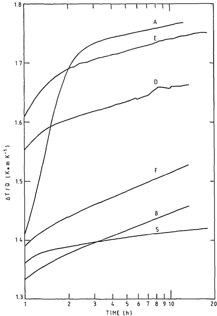
Figure 8 Temperature rise per unit power measured during the heating phase with the probe in various holes.
