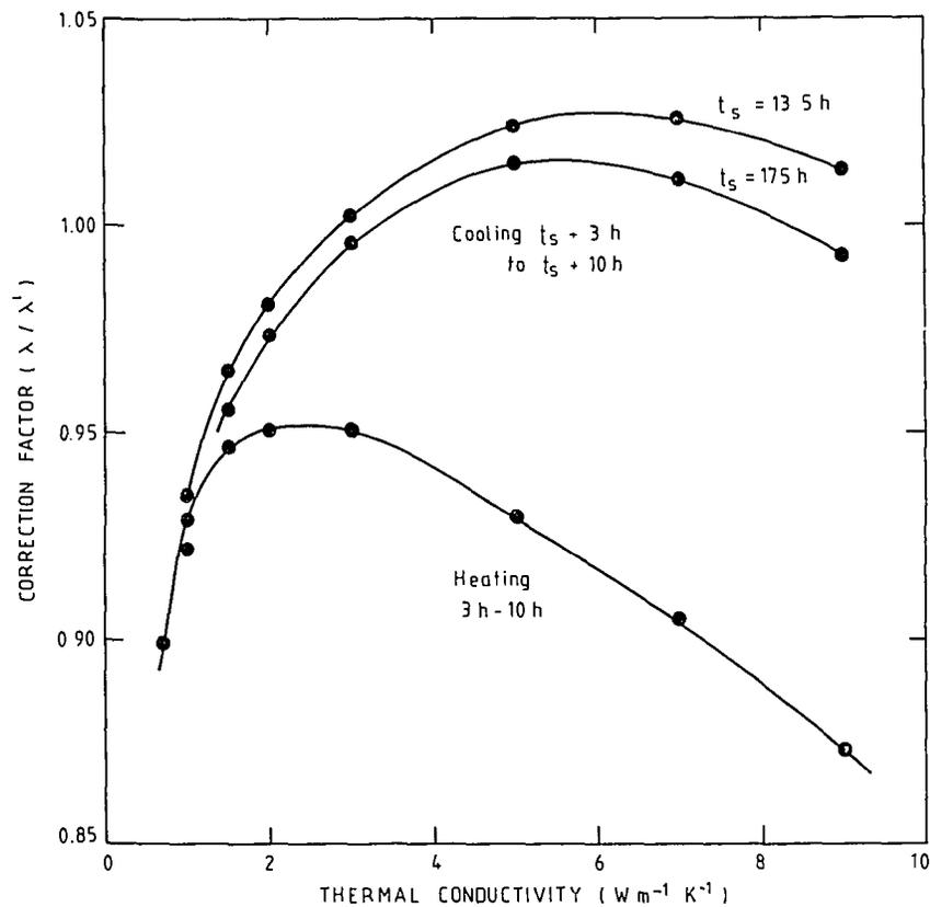
Figure 10 Correction factors calculated using HEATRAN for determining the thermal conductivity  $\lambda$  from the estimate  $\lambda'$  obtained by a least squares fit of the temperature data to equation 9 for an infinite line heat source. The correction factors shown for the cooling phase are for switch-off times of 13.5 and 17.5 hours.
