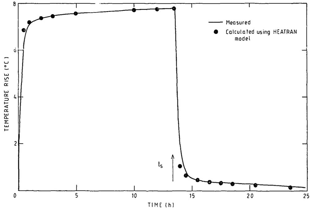
Figure 7 Probe temperatures in hole F compared to the temperatures calculated using HEATRAN with a thermal conductivity for the dump of  $1.75 \text{ W m}^{-1} \text{ K}^{-1}$ . The conductivity of the air boundary layer has been adjusted in the calculation so that the calculated temperatures agree with measurement after 3 hours of heating.
