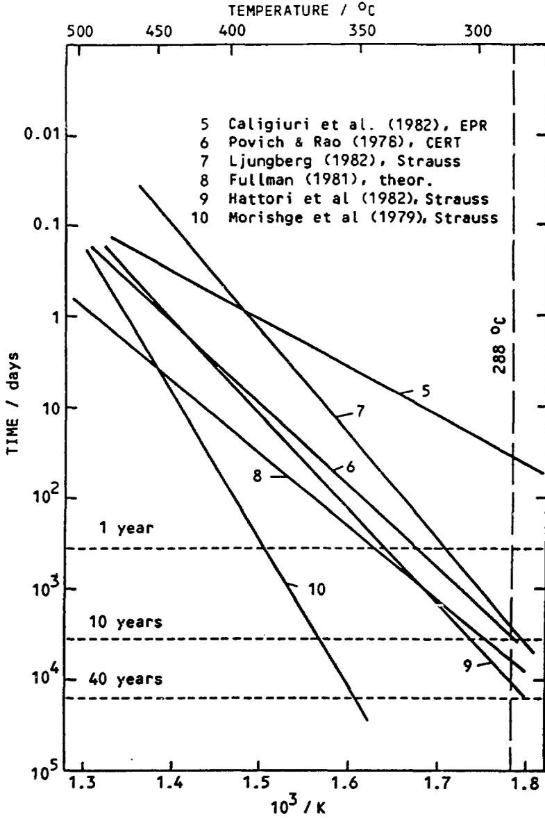
Fig. 5. Several (T, t) dependences for LTS of AISI 304 steel showing wide scatter of various tests. The scatter is based on the various starting conditions used as well as test methods (Kekkonen et al., 1984).
