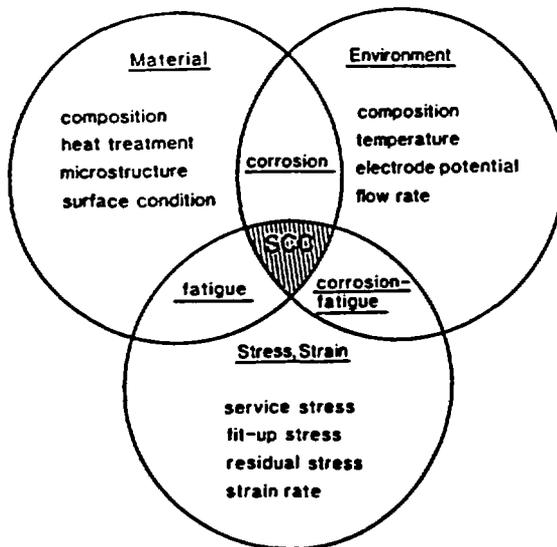
Fig. 1. Factors affecting environment sensitive cracking. Note that specific conditions are required for cracking to occur.
