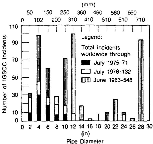
Fig. 4. World-wide frequency of BWR pipe cracking incidents as a function of pipe diameter (Danko, 1984).
