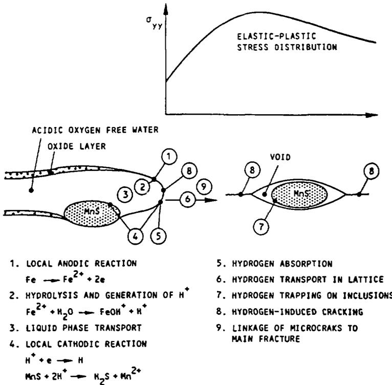
Fig. 3. Schematic illustration of effects of MnS-inclusions of the steel in cyclic crack growth of reactor pressure vessel steels in high-temperature, high-pressure reactor water (Hänninen et al., 1983).
