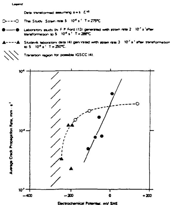
Fig. 6. Variation of average IGSCC crack propagation rate with corrosion potential for sensitized AISI 304 steel indicating a critical potential for IGSCC (Ljungberg and Korhonen, 1984).
