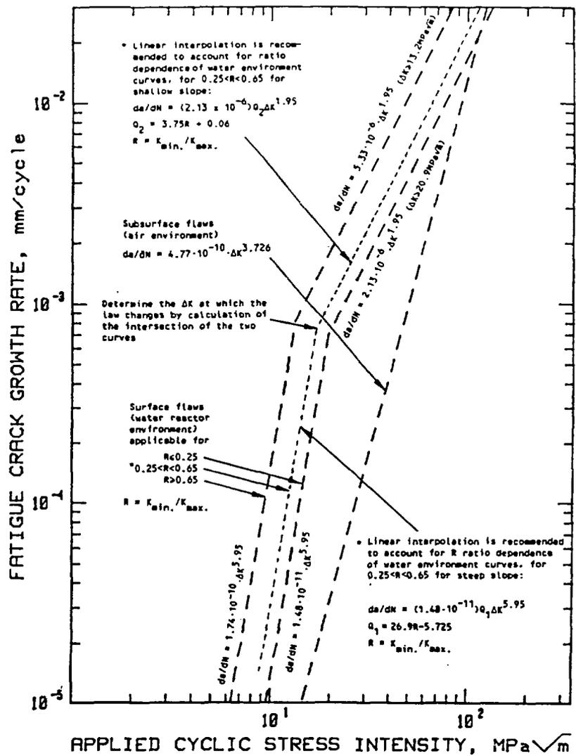
Fig. 2. The ASME Code crack growth rate reference curves for reactor pressure vessel steels.
