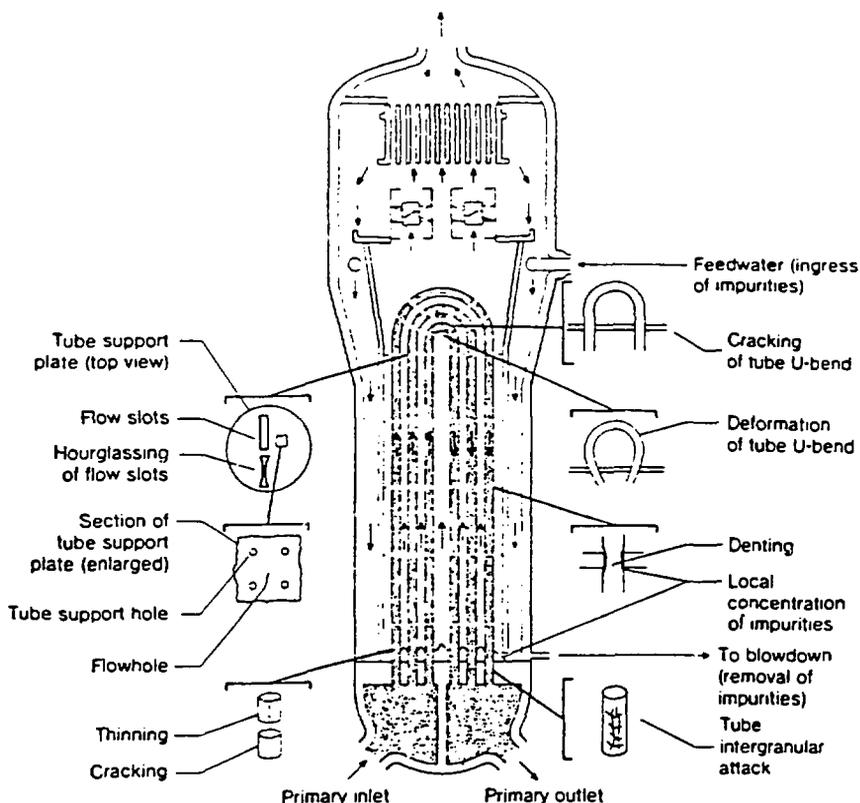
Fig. 8. Schematic picture of a recirculating steam generator with problem areas, where many, but not all units, have had various forms of corrosion (Green and Paine, 1981).
