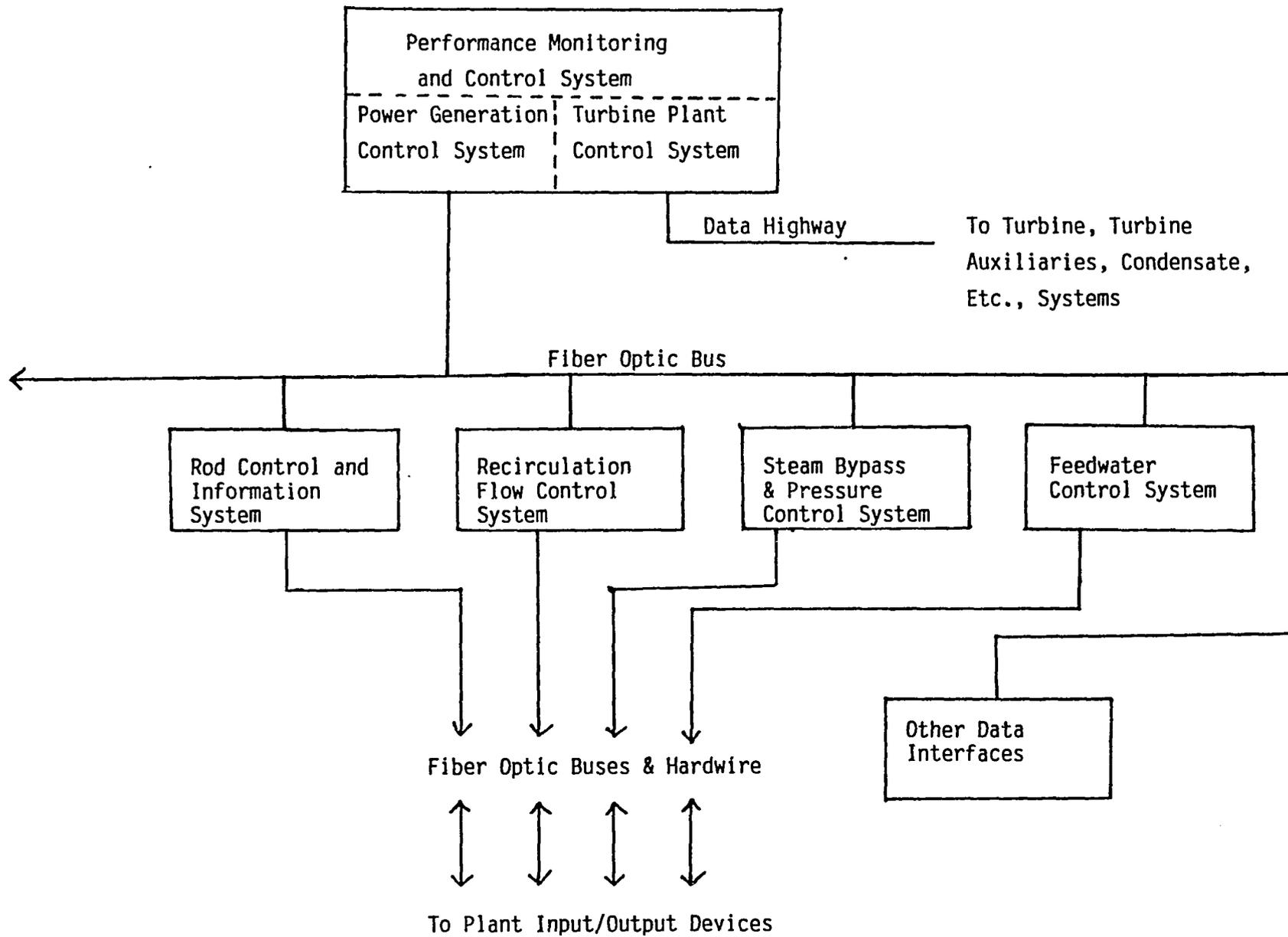
Figure 1. ABWR "Hierarchical Distributed Architecture"
