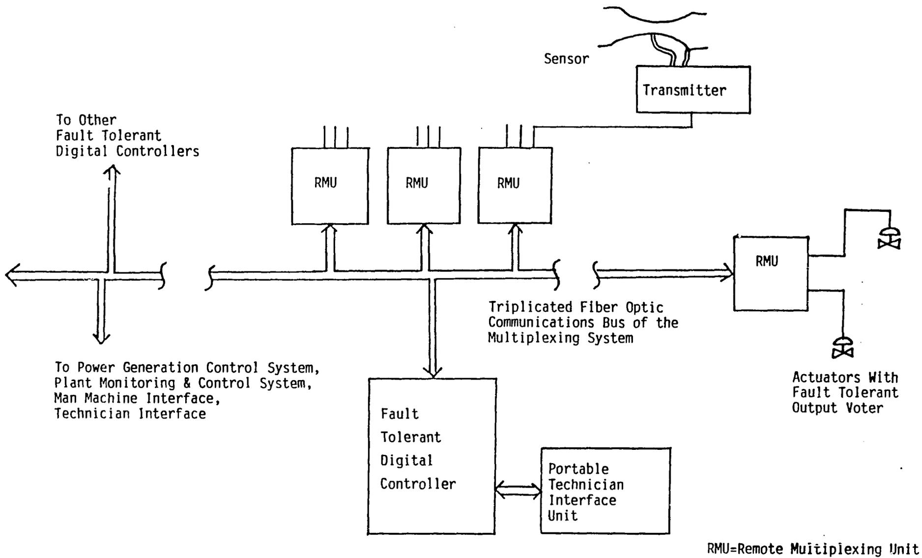
Figure 6. ABWR Process Control Configuration
