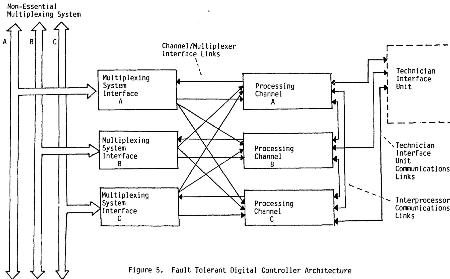
Figure 5. Fault Tolerant Digital Controller Architecture
