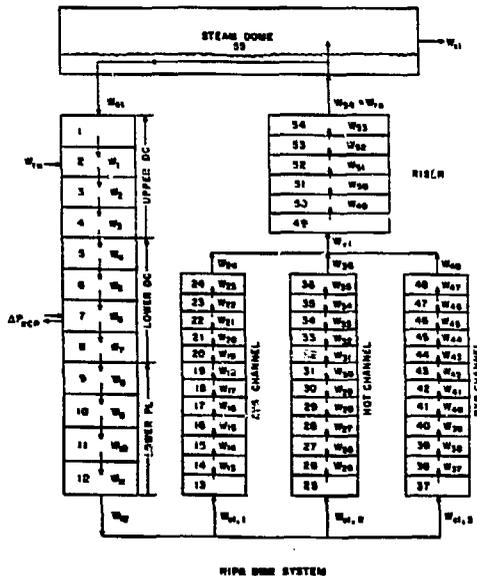
Figure 5 Nodalization Scheme for Pressure Vessel
