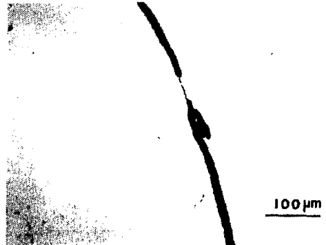
FIGURE 7 TYPICAL LEAK PATH DUE TO INCOMPLETE SHEATH TO END-CAP CLOSURE WELD. MICROGRAPH OF WELD INTER-FACE.
