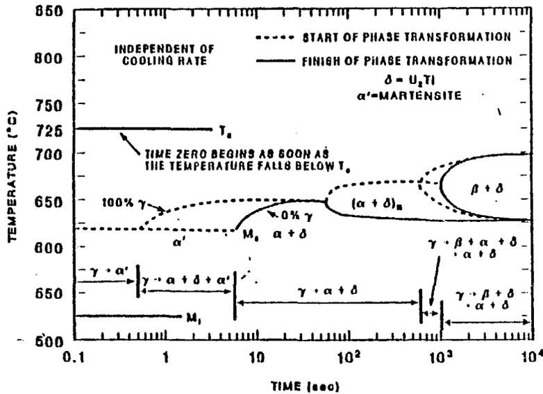
Fig. 1. Phases of U-0.75Ti alloy as functions of time and temperature for continuous cooling.
