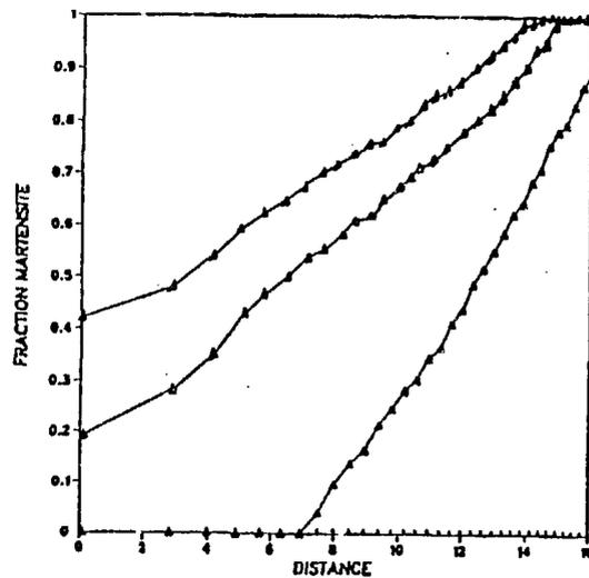
Fig. 7. Fraction of martensite at the final time as a function of film heat transfer coefficient (Cases 7, 8, and 9).
