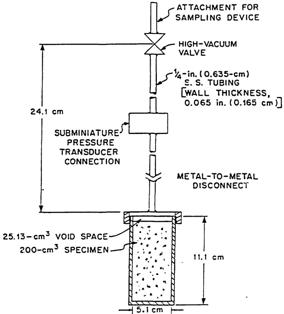
FIG. 2 — Alpha- and gamma-radiolysis specimen holder and pressure-measuring equipment for the 200-cm<sup>3</sup> specimens of cured grouts with simulated current acid waste (CAW) and double-shell slurry (DSS) radioactive waste streams.
