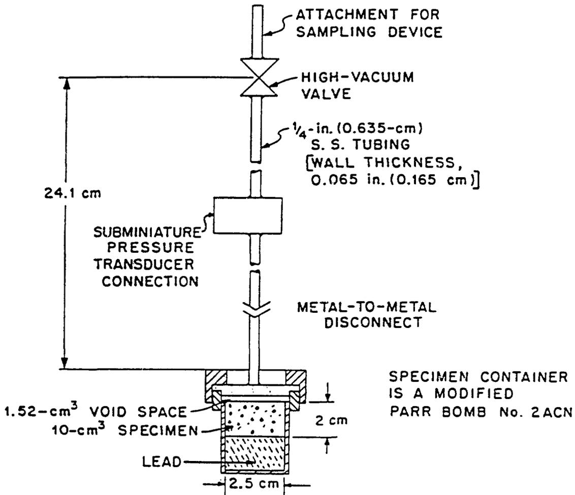
FIG. 1 — Alpha- and gamma-radiolysis specimen holder and pressure-measuring equipment for the 10-cm<sup>3</sup> specimens of cured grouts with simulated current acid-waste (CAW) and double-shell slurry (DSS) radioactive waste streams.
