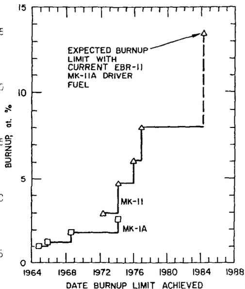
Figure 2--EBR-II Driver Fuel Burnup Capability.
