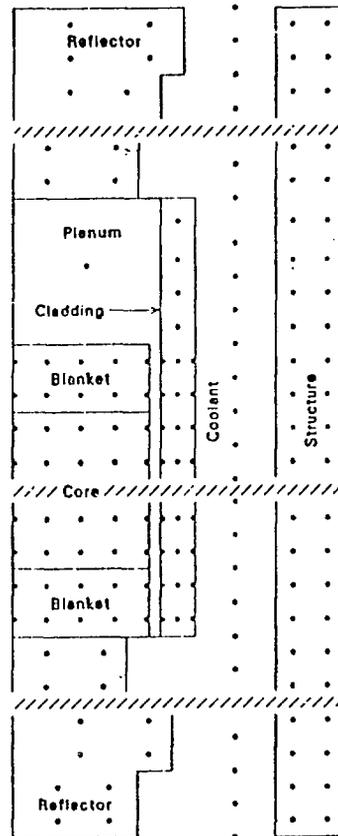
Fig. 1. SAS4A/DEFORM-4 Node Structure.
