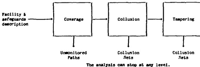
Fig. 1. Stages of an SAA physical security vulnerability assessment.
