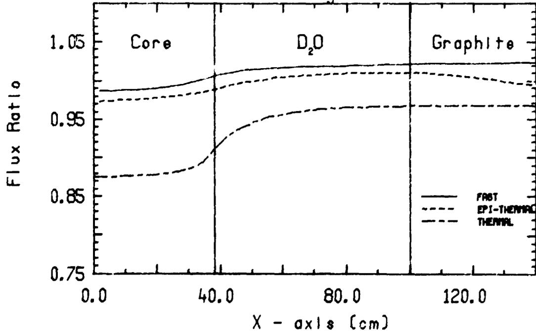
Figure B-3. Flux Ratios at Core Mid-plane
