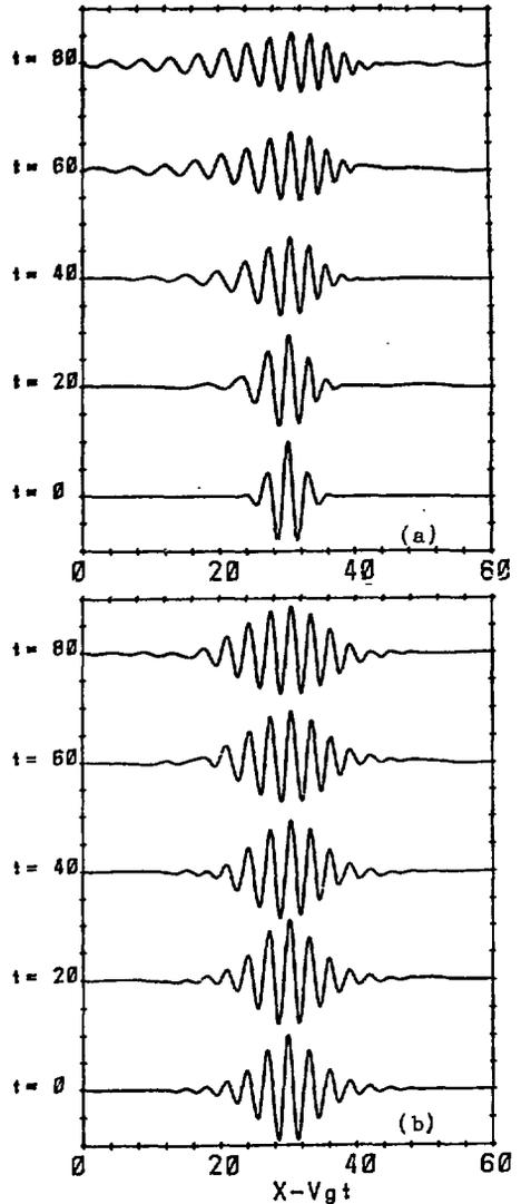
Fig.1 Propagation of a wave packet (a) and an envelope soliton (b), where  $k = 2/3\pi$ ,  $|\phi|^2 = 0.01$
